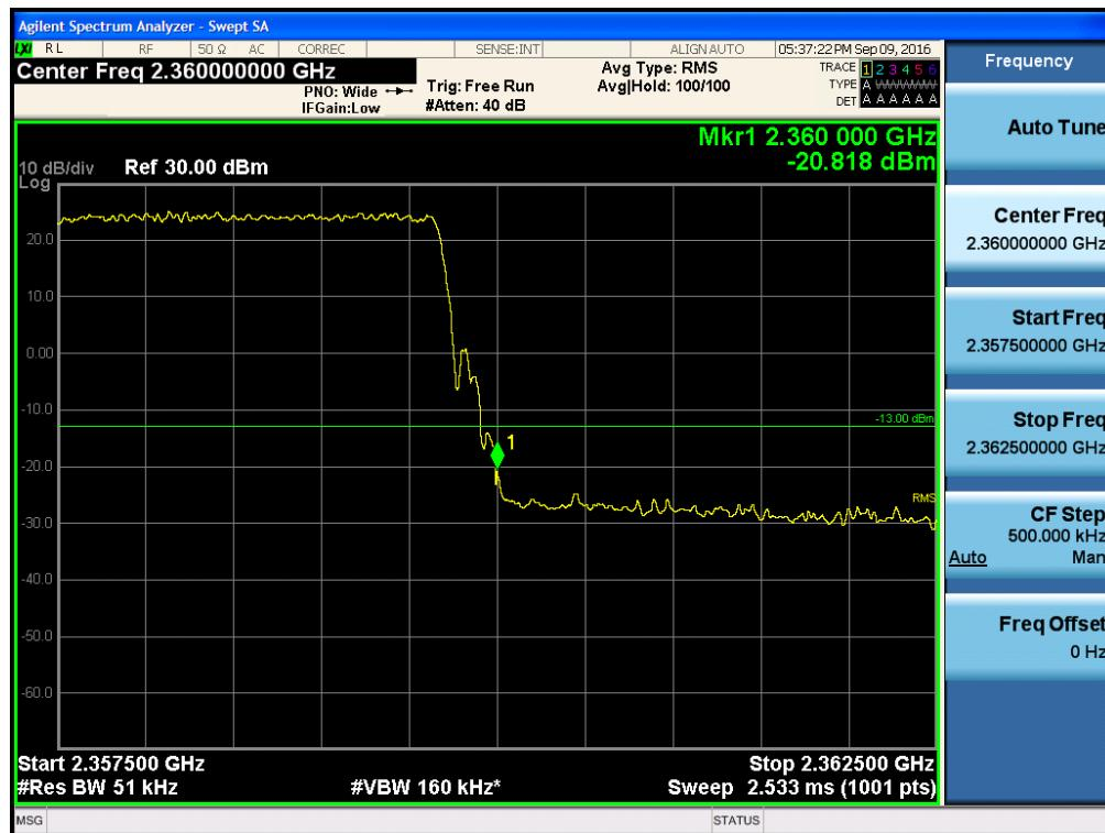
**Single channel Enhancer Band Edge\_2300\_WCS BAND LTE 10 MHz**
