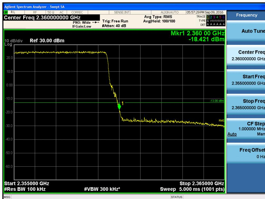
**Intermodulation Spurious Emissions for FCC\_2300\_WCS BAND LTE 5 MHz**
