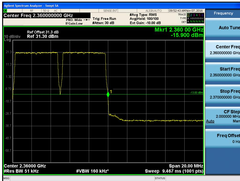
**Intermodulation Spurious Emissions for FCC\_2300\_WCS BAND LTE 10 MHz**
