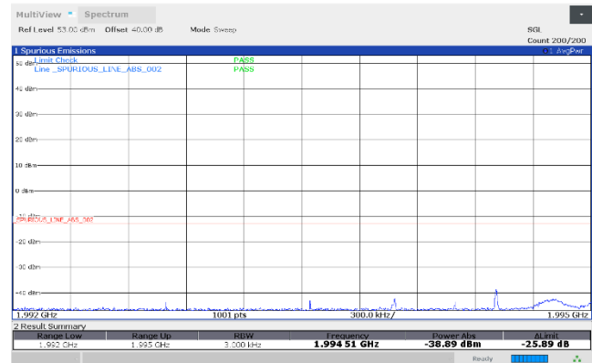
Low band edge, 1 signal, total level = 0.5 dB less than AGC threshold
