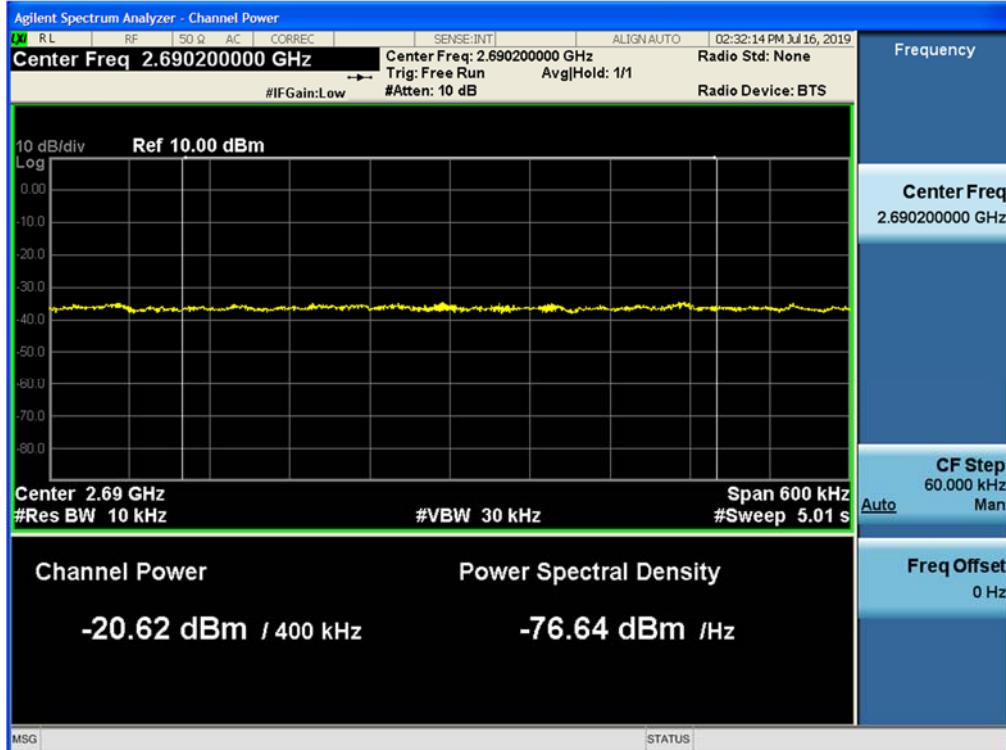
**+3 dB above Out-of-band (single test signal) / BRS/EBS 5G NR / Downlink / NR 40 MHz / Lower**
