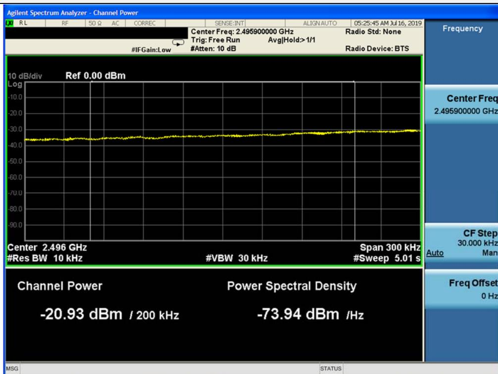
+3 dB above Out-of-band (two adjacent test signals) / BRS/EBS 5G NR / Downlink / NR 40 MHz / Upper
