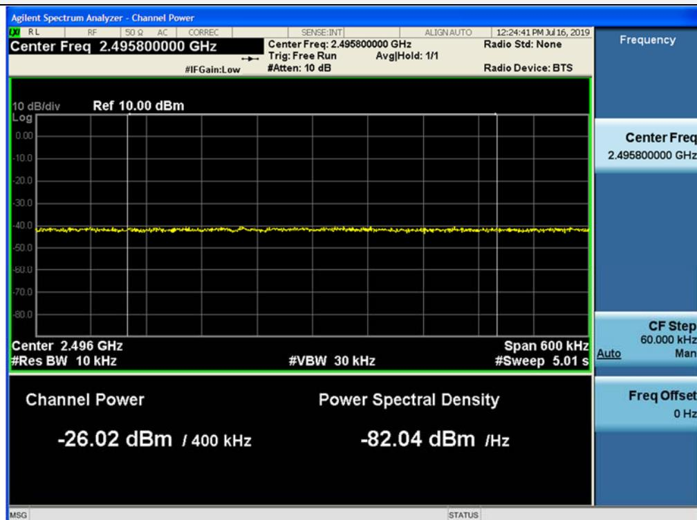
+3 dB above Out-of-band (two adjacent test signals) / BRS/EBS 5G NR / Downlink / NR 60 MHz / Upper
