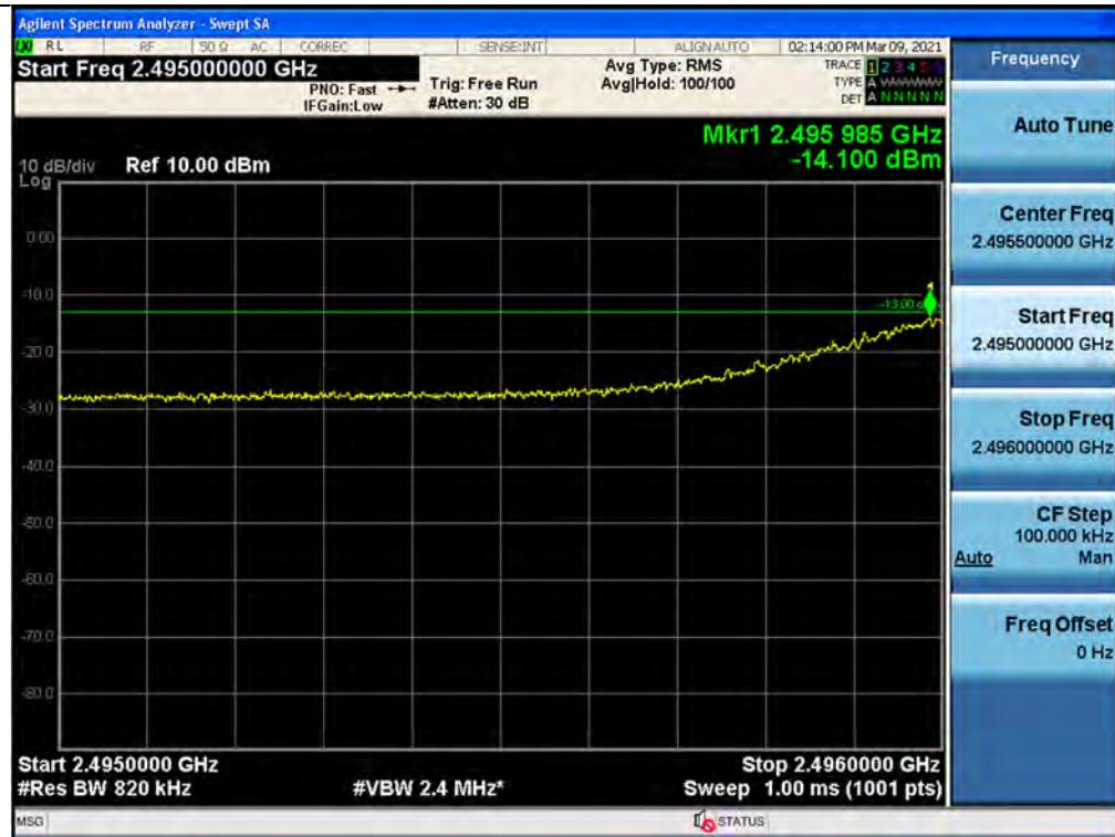
+3 dB above Out-of-band (single test signals) / BRS/EBS / Downlink / 5G NR 80 MHz / Upper
