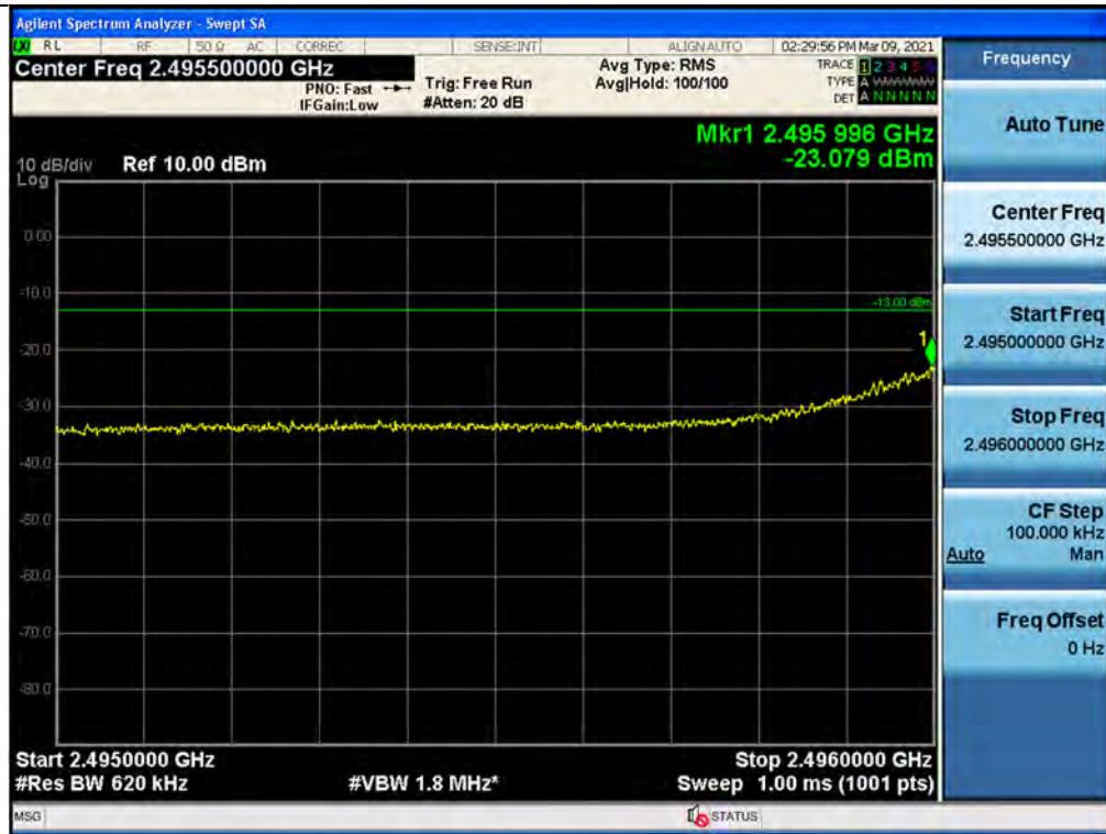
+3 dB above Out-of-band (two adjacent test signals) / BRS/EBS / Downlink / 5G NR 60 MHz / Upper
