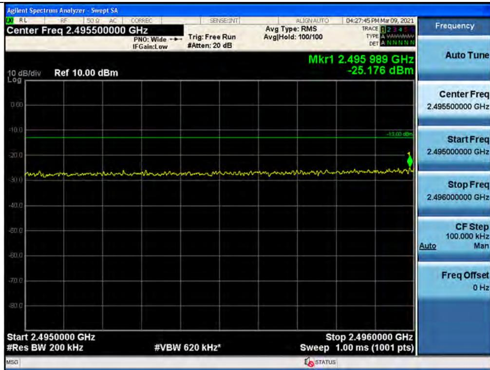
+3 dB above Out-of-band (two adjacent test signals) / BRS/EBS / Downlink / LTE 20 MHz / Upper
