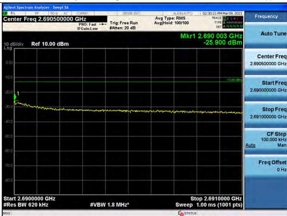
+3 dB above Out-of-band (two adjacent test signals) / BRS/EBS / Downlink / 5G NR 60 MHz / Lower
