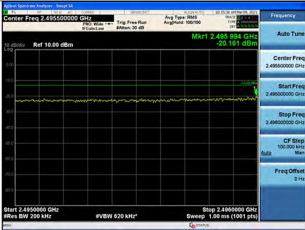
+3 dB above Out-of-band (single test signals) / BRS/EBS / Downlink / LTE 20 MHz / Upper
