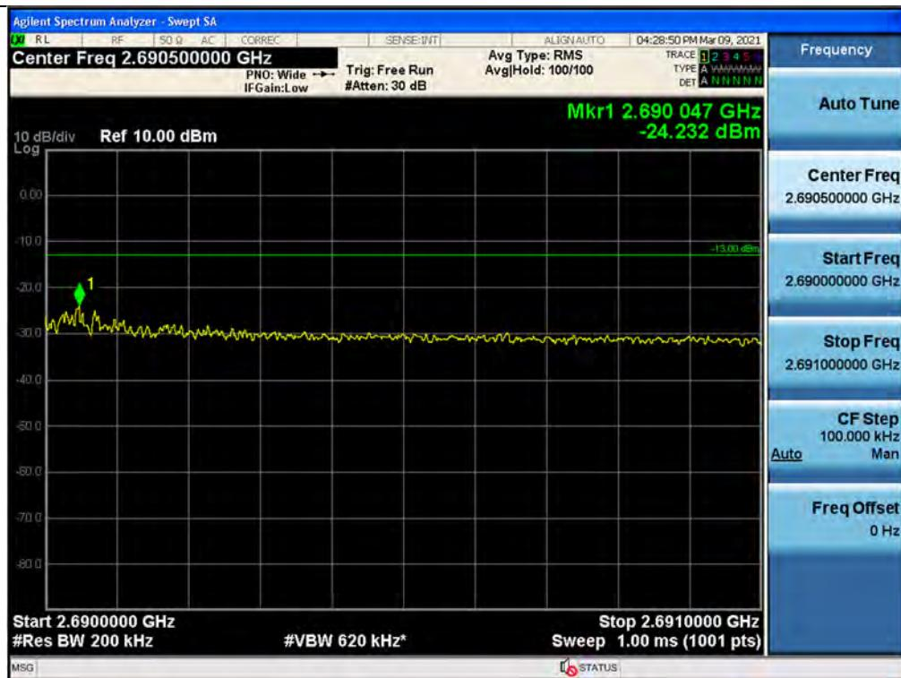
+3 dB above Out-of-band (single test signals) / BRS/EBS / Downlink / LTE 20 MHz / Lower
