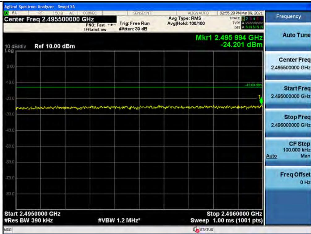
+3 dB above Out-of-band (single test signals) / BRS/EBS / Downlink / 5G NR 40 MHz / Upper
