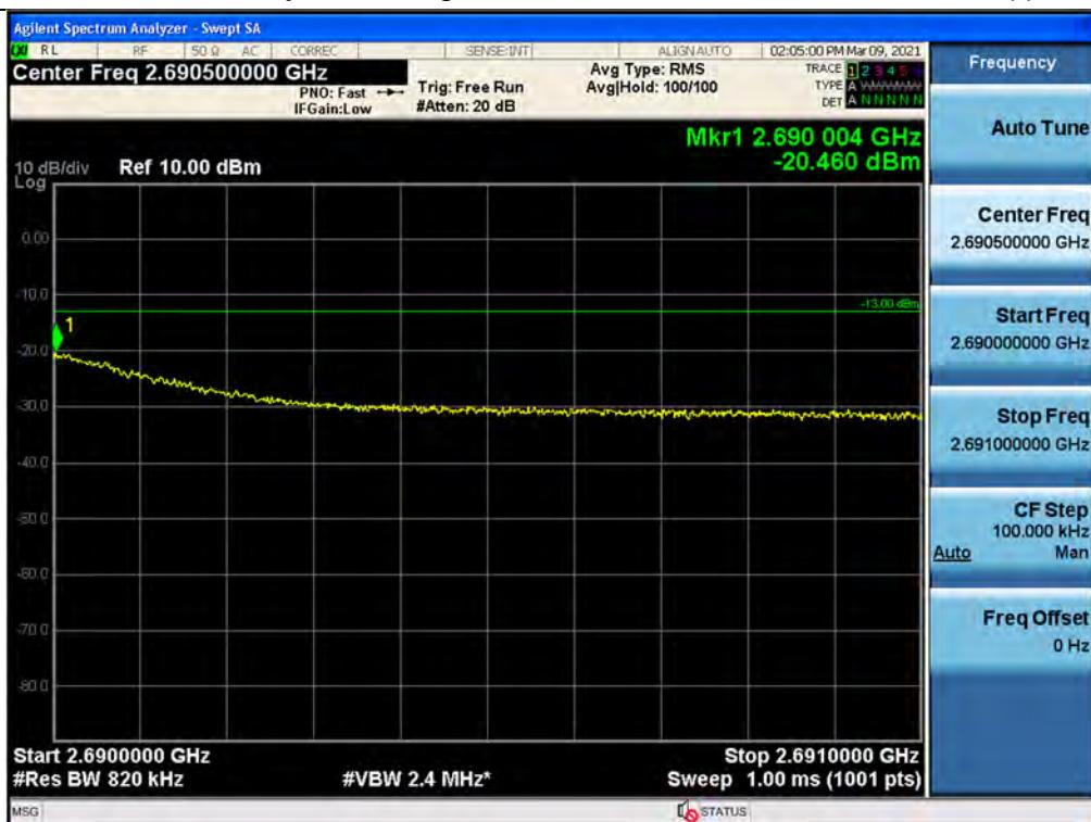
+3 dB above Out-of-band (two adjacent test signals) / BRS/EBS / Downlink / 5G NR 80 MHz / Lower
