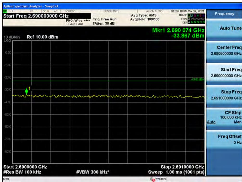
+3 dB above Out-of-band (single test signals) / BRS/EBS / Downlink / 5G NR 100 MHz / Lower
