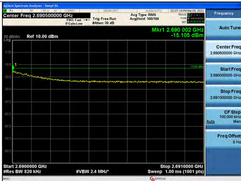
+3 dB above Out-of-band (single test signals) / BRS/EBS / Downlink / 5G NR 80 MHz / Lower
