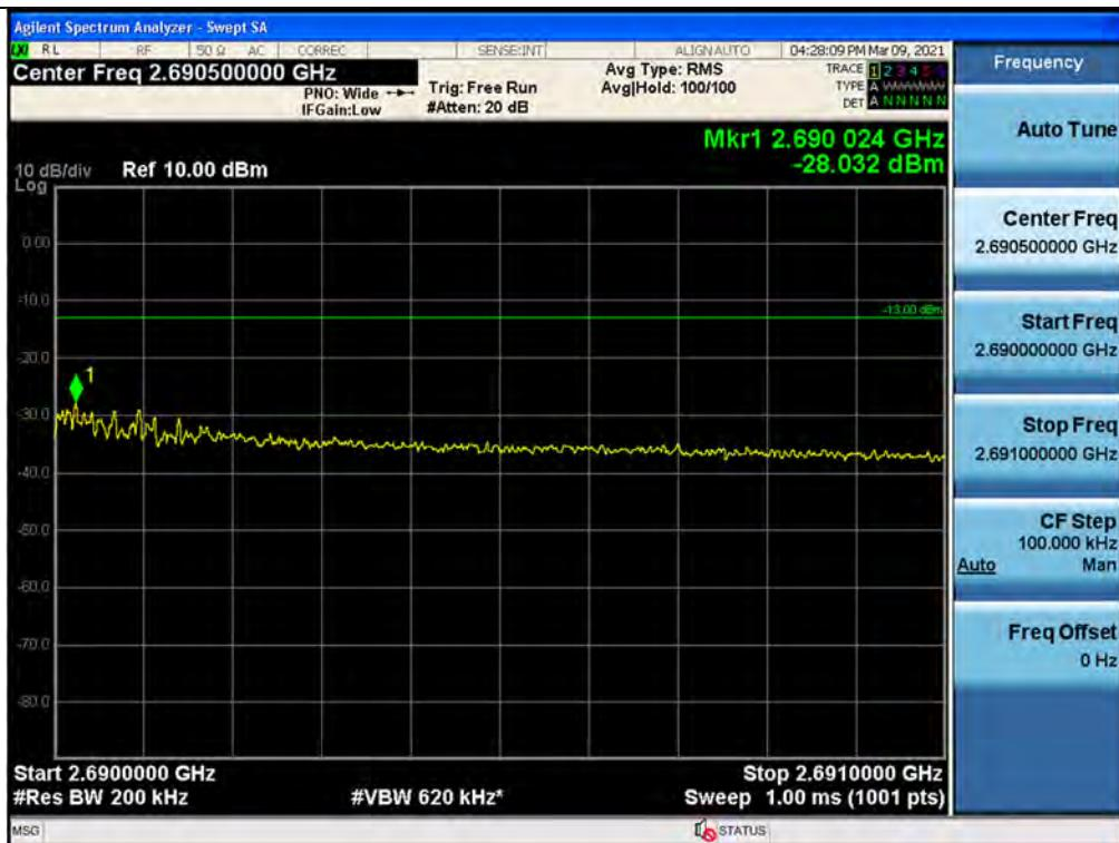
+3 dB above Out-of-band (two adjacent test signals) / BRS/EBS / Downlink / LTE 20 MHz / Lower
