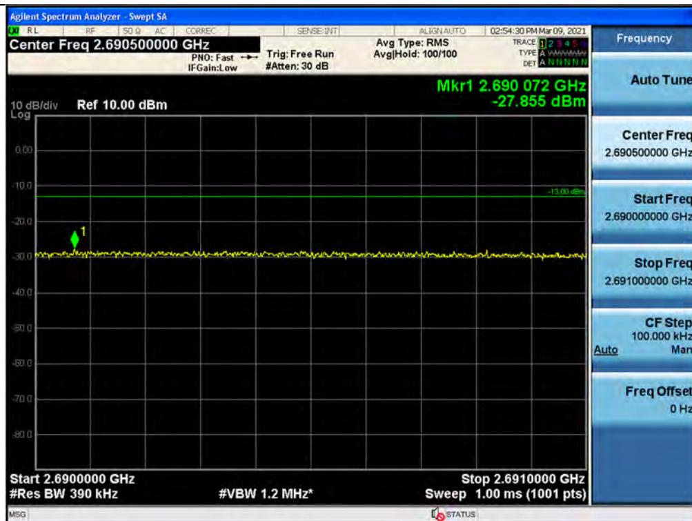
+3 dB above Out-of-band (single test signals) / BRS/EBS / Downlink / 5G NR 40 MHz / Lower
