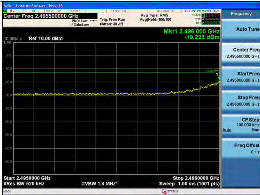
+3 dB above Out-of-band (single test signals) / BRS/EBS / Downlink / 5G NR 60 MHz / Upper
