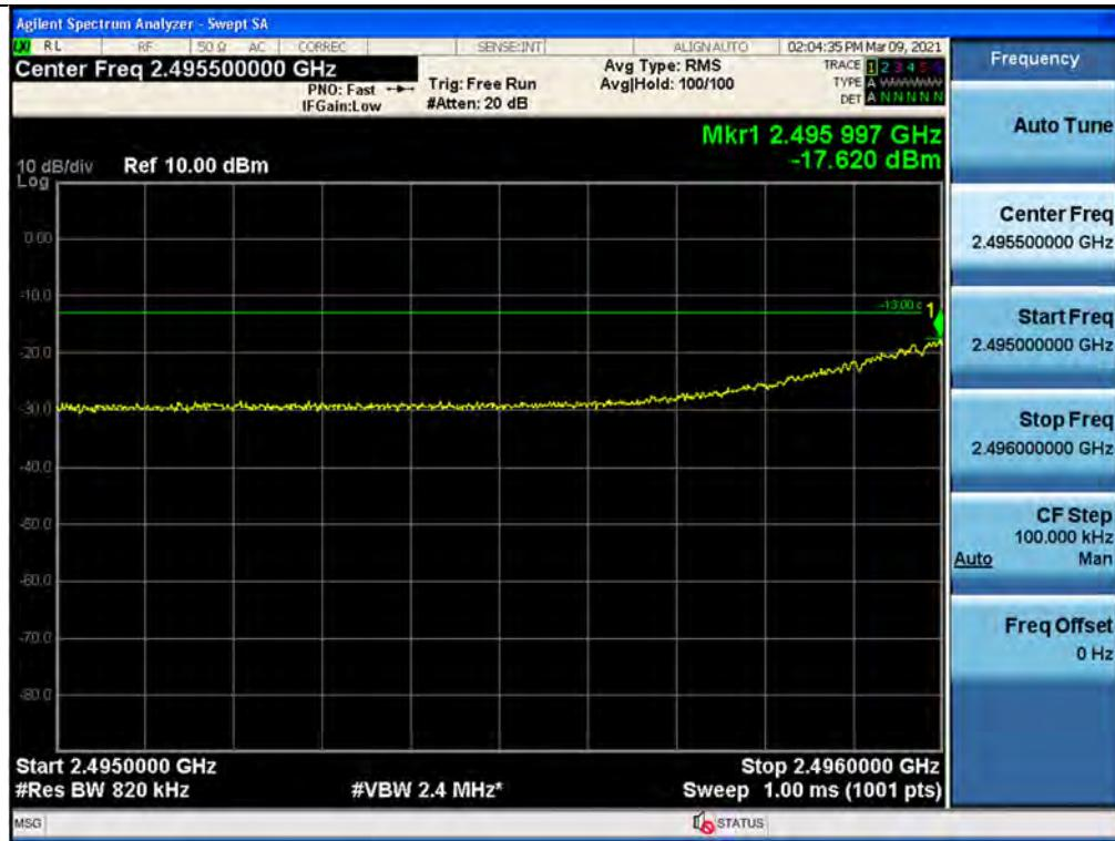
+3 dB above Out-of-band (two adjacent test signals) / BRS/EBS / Downlink / 5G NR 80 MHz / Upper
