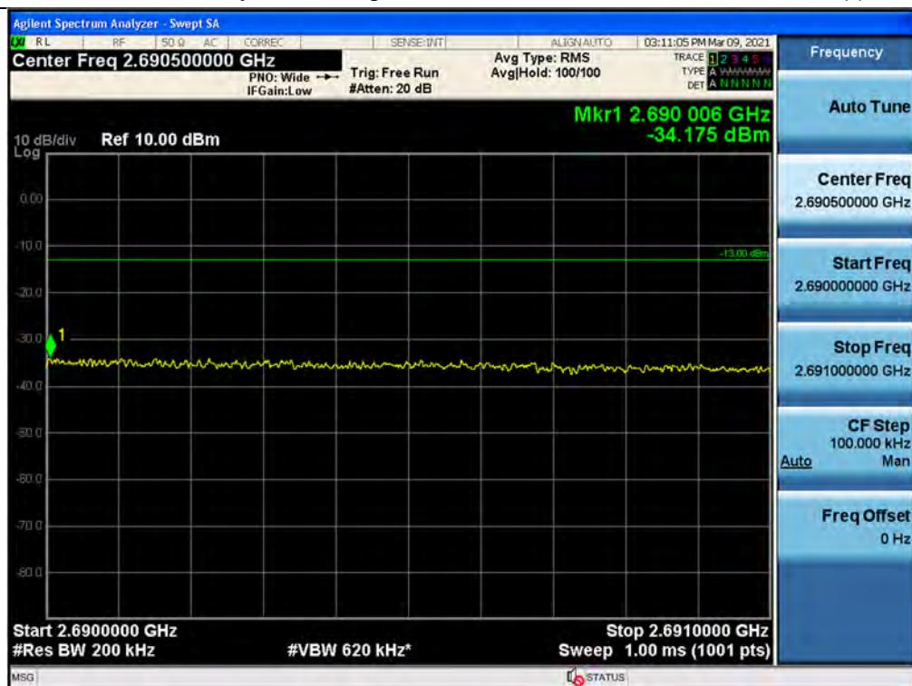
+3 dB above Out-of-band (two adjacent test signals) / BRS/EBS / Downlink / 5G NR 20 MHz / Lower
