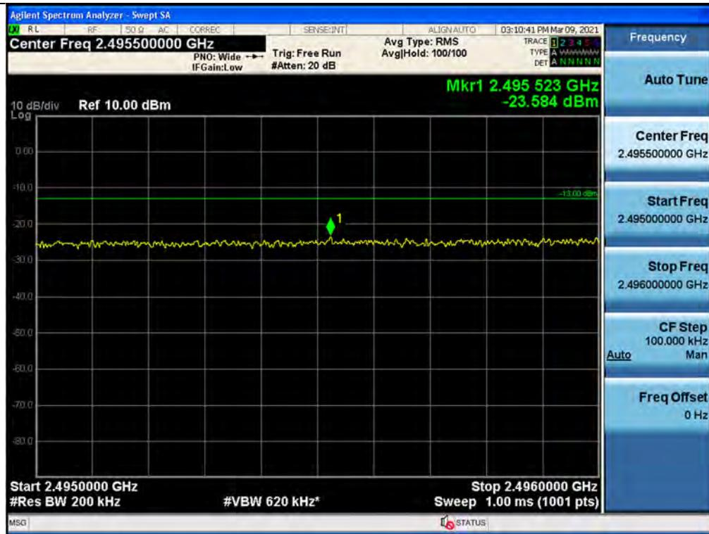
+3 dB above Out-of-band (two adjacent test signals) / BRS/EBS / Downlink / 5G NR 20 MHz / Upper
