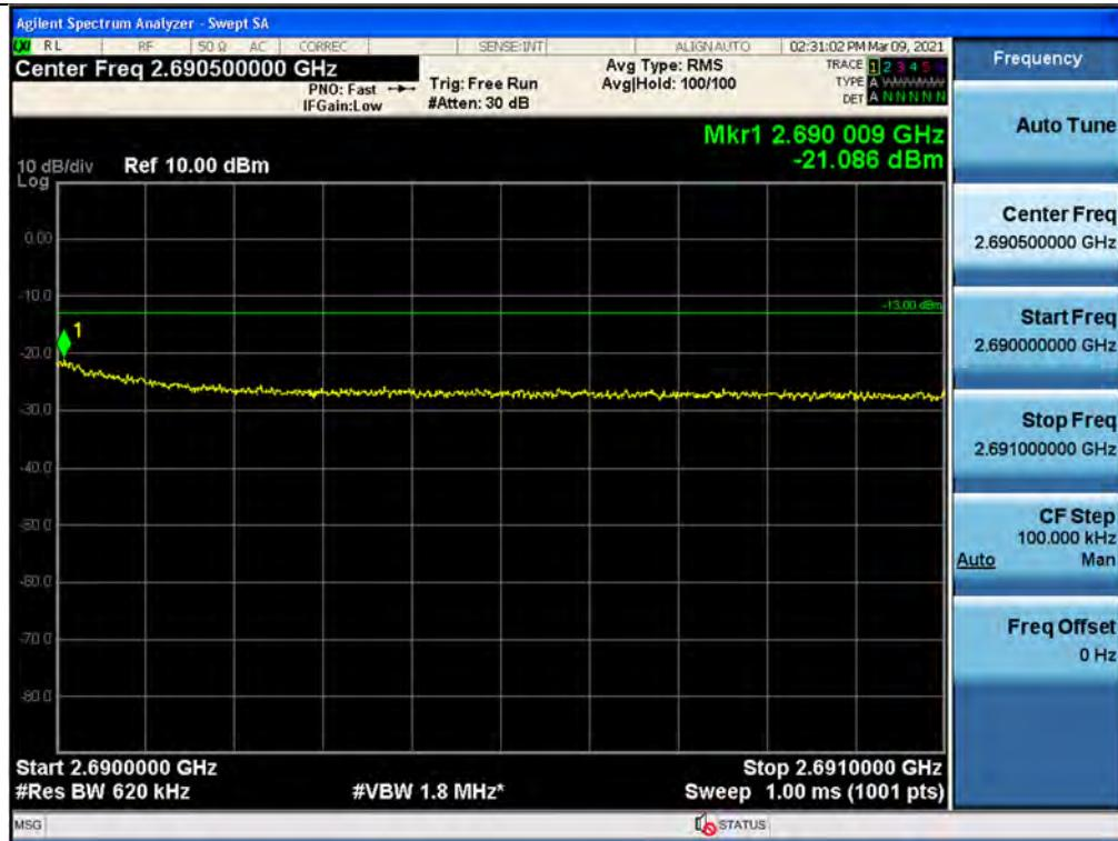
+3 dB above Out-of-band (single test signals) / BRS/EBS / Downlink / 5G NR 60 MHz / Lower
