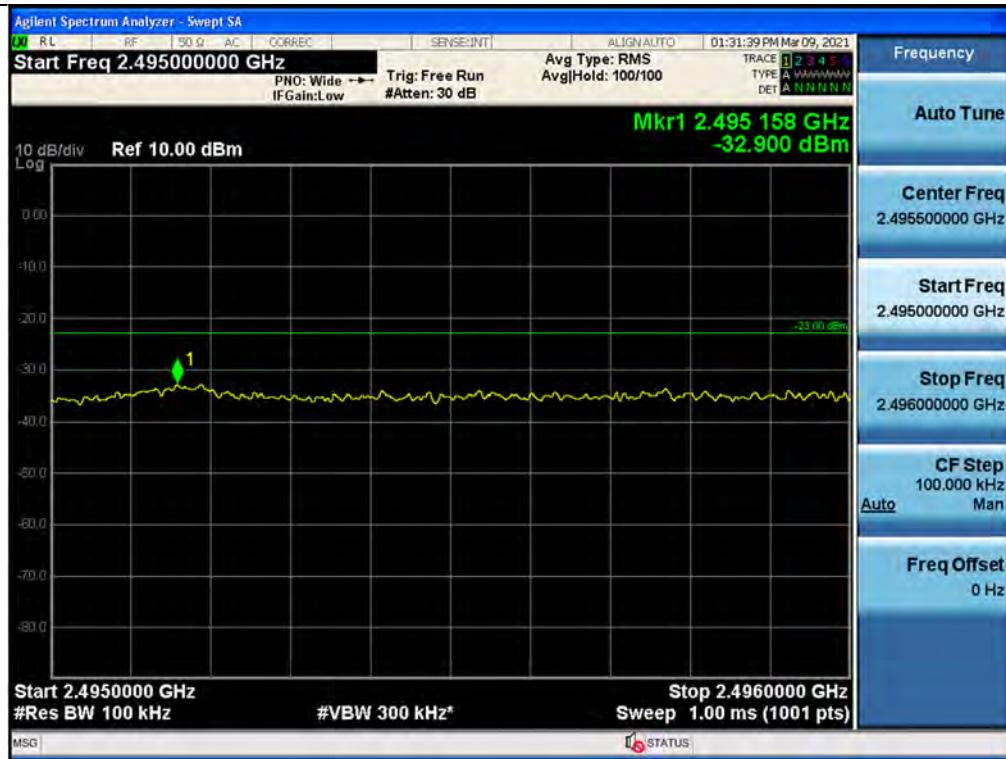
+3 dB above Out-of-band (single test signals) / BRS/EBS / Downlink / 5G NR 100 MHz / Upper
