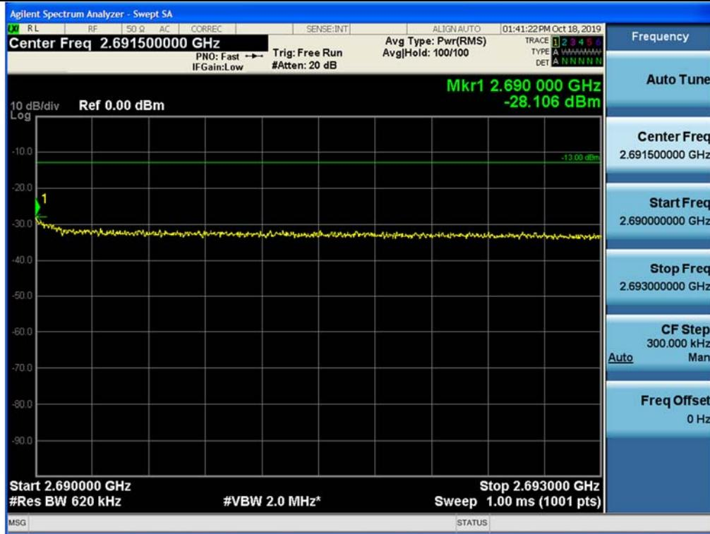
+3 dB above Out-of-band (single test signal) / Broadband PCS 5G NR / Downlink / NR 60 MHz / Lower
