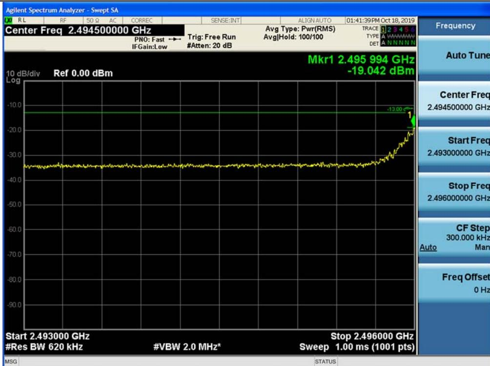
+3 dB above Out-of-band (single test signal) / Broadband PCS LTE 20M / Downlink / LTE 20 MHz / Upper
