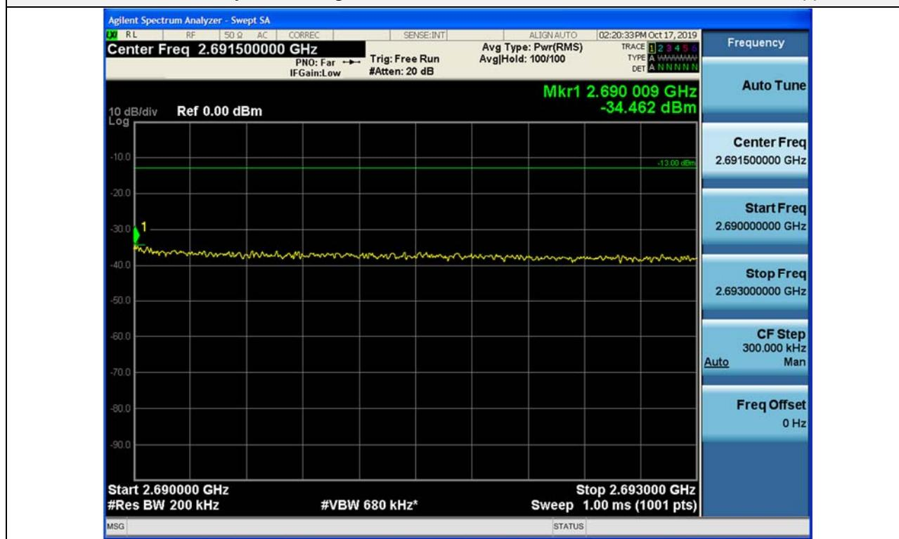
Out-of-band (two adjacent test signals) / Broadband PCS LTE 20M / Downlink / LTE 20 MHz / Lower
