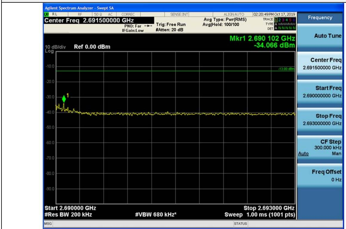
+3 dB above Out-of-band (two adjacent test signals) / Broadband PCS LTE 20M / Downlink / LTE 20 MHz / Lower
