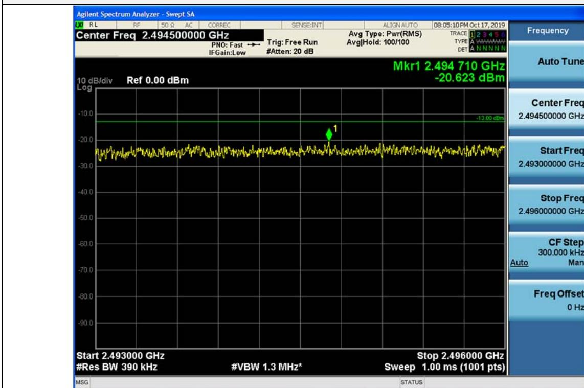
+3 dB above Out-of-band (single test signal) / Broadband PCS 5G NR / Downlink / NR 60 MHz / Upper
