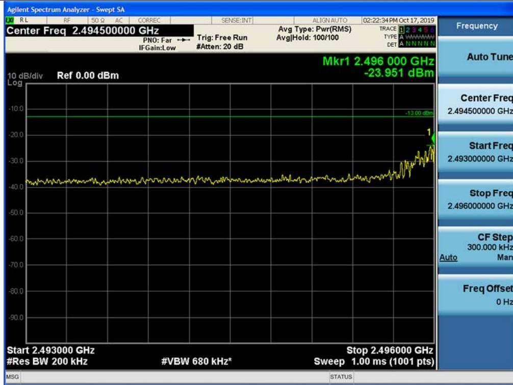
+3 dB above Out-of-band (single test signal) / Broadband PCS 5G NR / Downlink / NR 40 MHz / Upper
