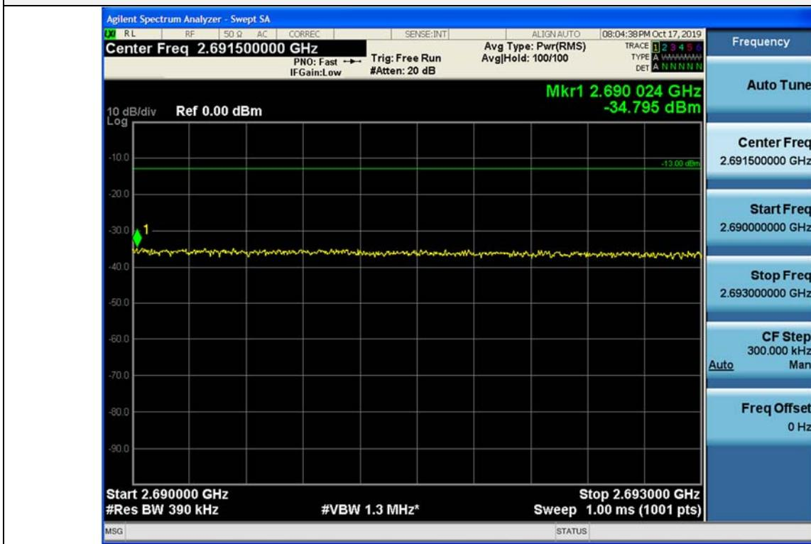
+3 dB above Out-of-band (single test signal) / Broadband PCS 5G NR / Downlink / NR 40 MHz / Lower
