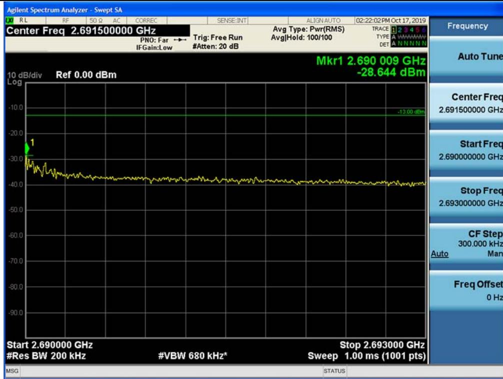
+3 dB above Out-of-band (single test signal) / Broadband PCS LTE 20M / Downlink / LTE 20 MHz / Lower
