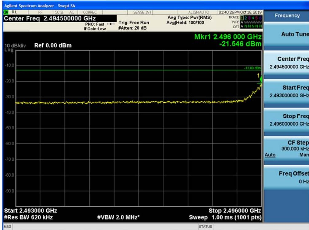
+3 dB above Out-of-band (two adjacent test signals) / Broadband PCS LTE 20M / Downlink / LTE 20 MHz / Upper
