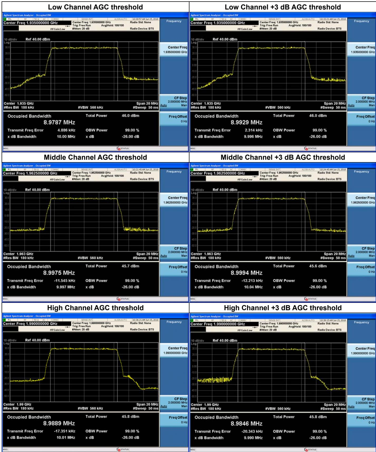
**Plots of Output Occupied Bandwidth for 1900 PCS Band LTE 20 MHz**
