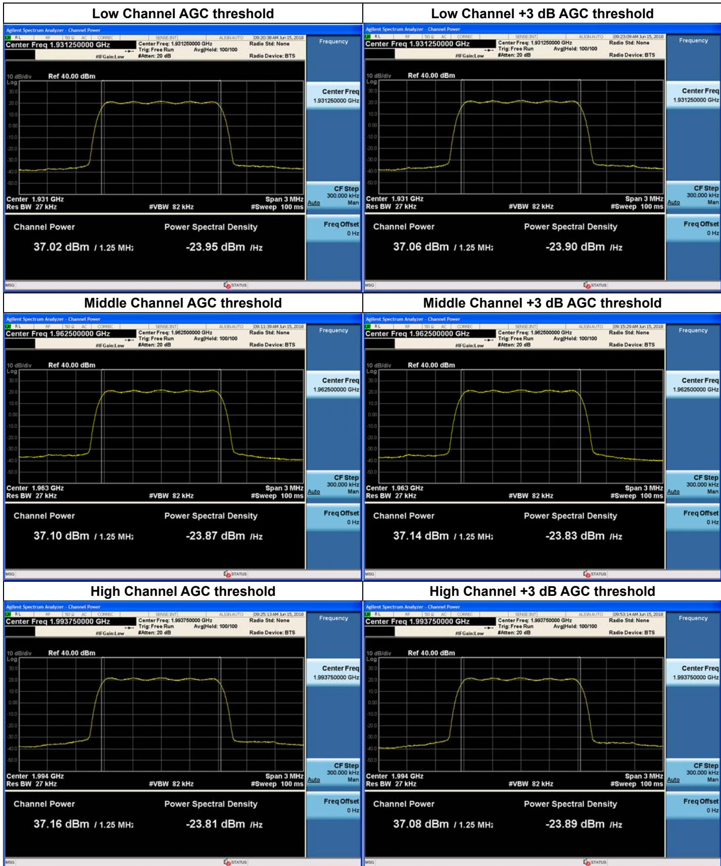
**Plots of RF Output Power for 1900 PCS Band GSM**
