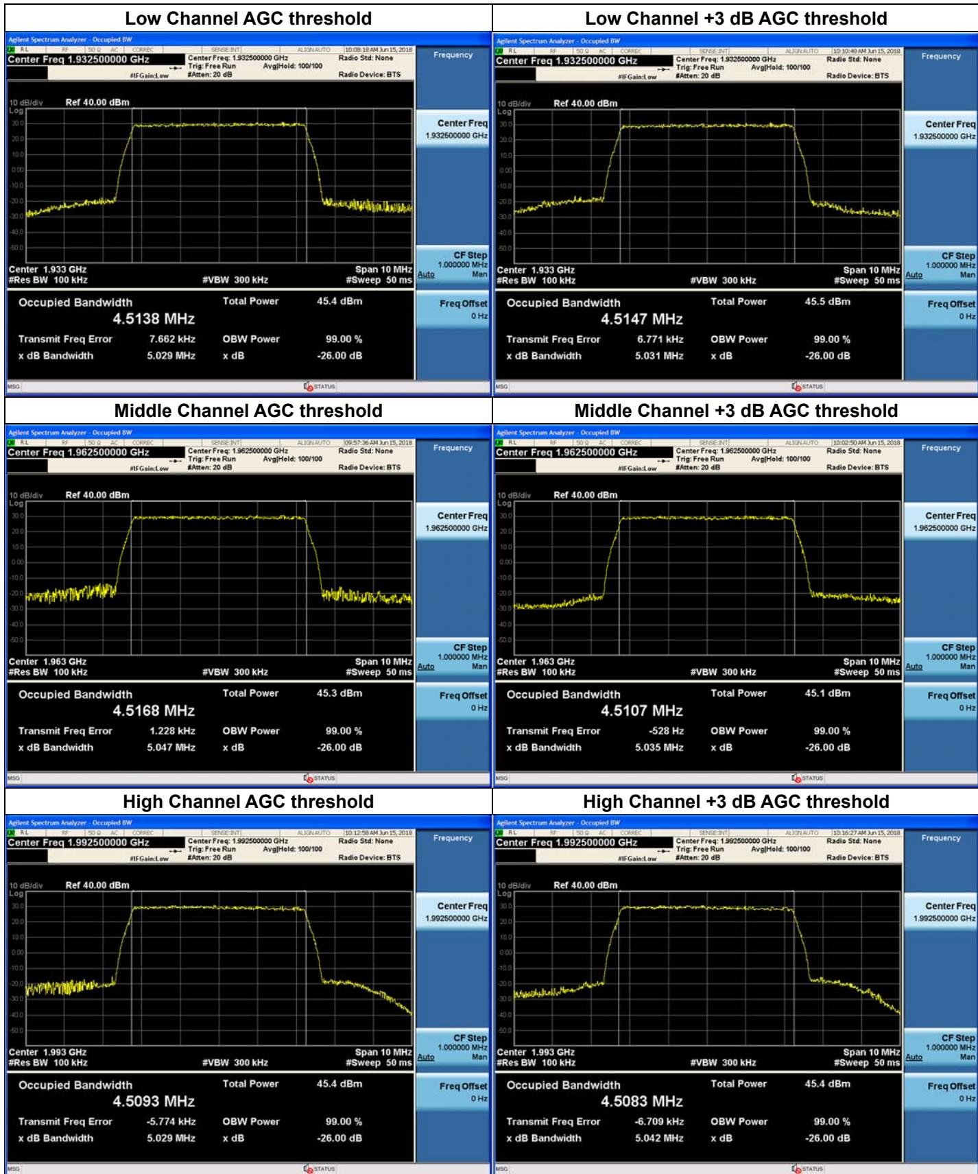
**Plots of Output Occupied Bandwidth for 1900 PCS Band LTE 10 MHz**
