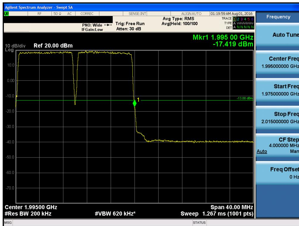
**Intermodulation Spurious Emissions for FCC\_1900 PCSBAND LTE 20 MHz**
