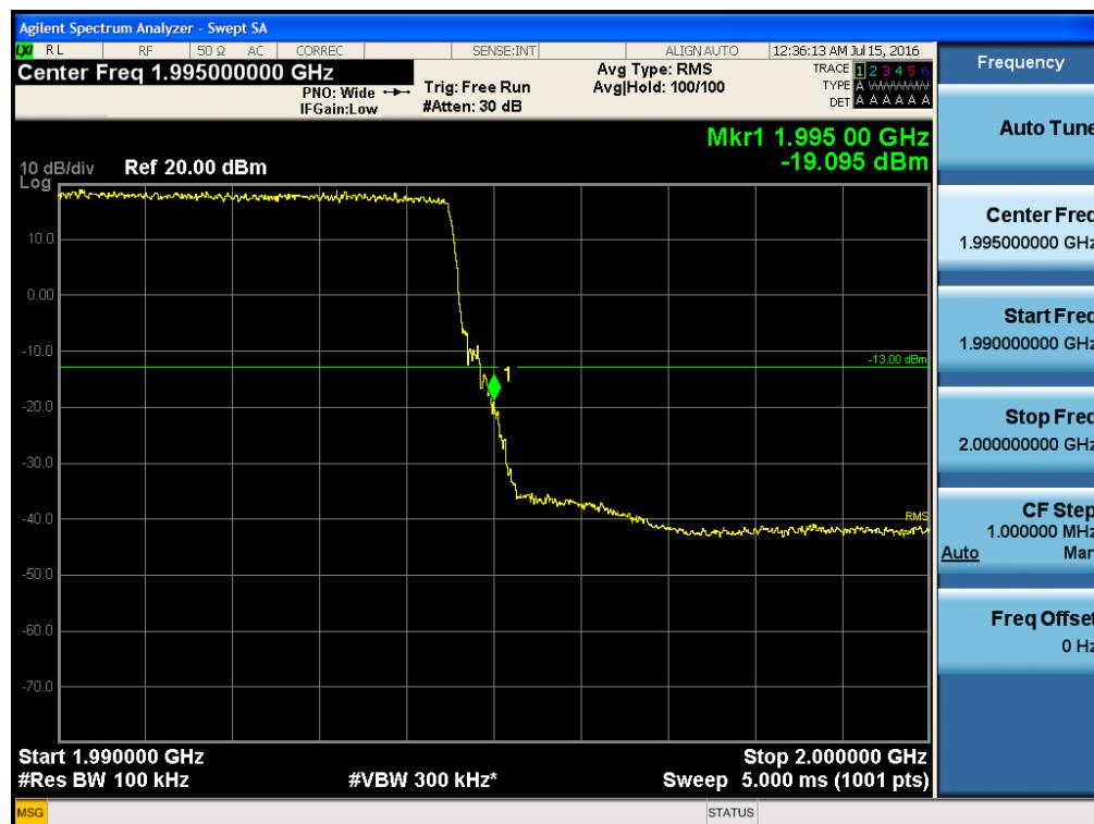
**Single channel Enhancer Band Edge\_1900 PCS BAND LTE 20 MHz**
