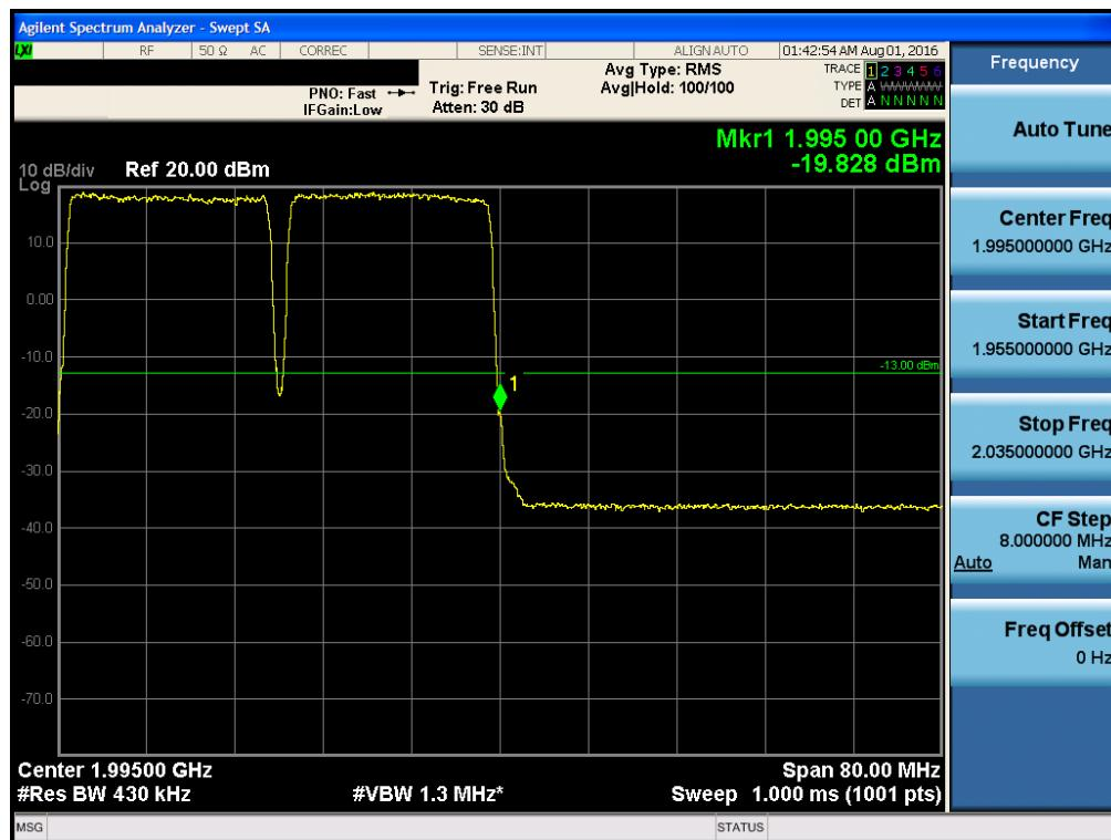
**Intermodulation Spurious Emissions for FCC\_1900 PCS CDMA**
