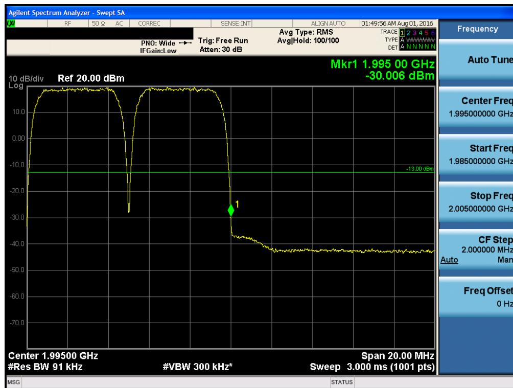
**Single channel Enhancer Band Edge\_1900 PCS13 BAND LTE 5 MHz**
