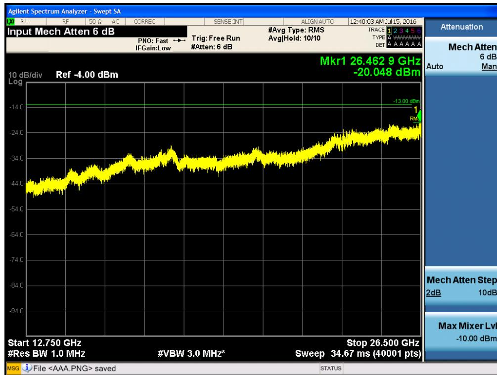
**Single channel Enhancer Plots of Spurious Emission for 1900 PCS BAND LTE 20 MHz
