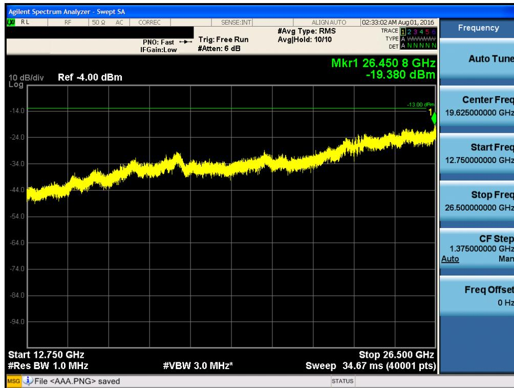
**Intermodulation Spurious Emissions for FCC\_1900 PCSBAND LTE 5 MHz**
