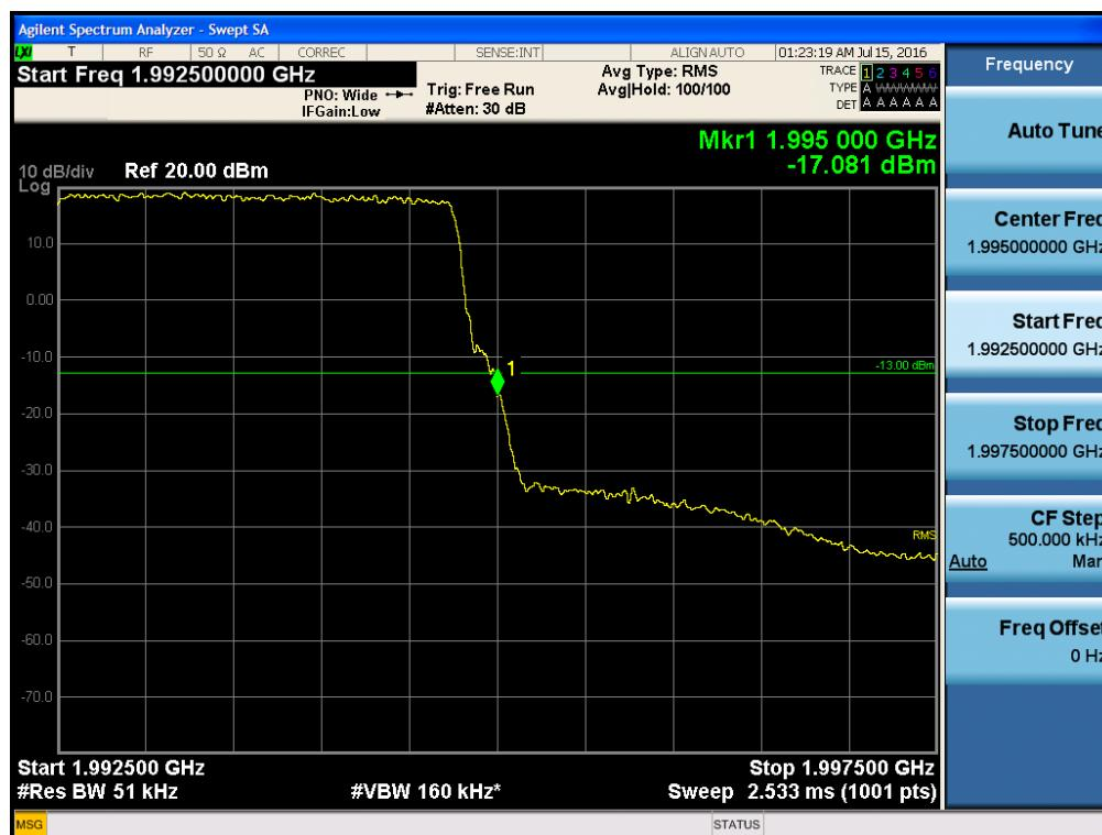
**Single channel Enhancer Band Edge\_1900 PCS13 BAND LTE 10 MHz**
