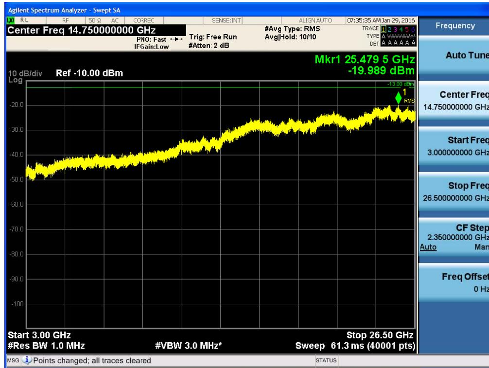
**Single channel Enhancer Plots of Spurious Emission for PCS1900 BAND LTE 10MHz
