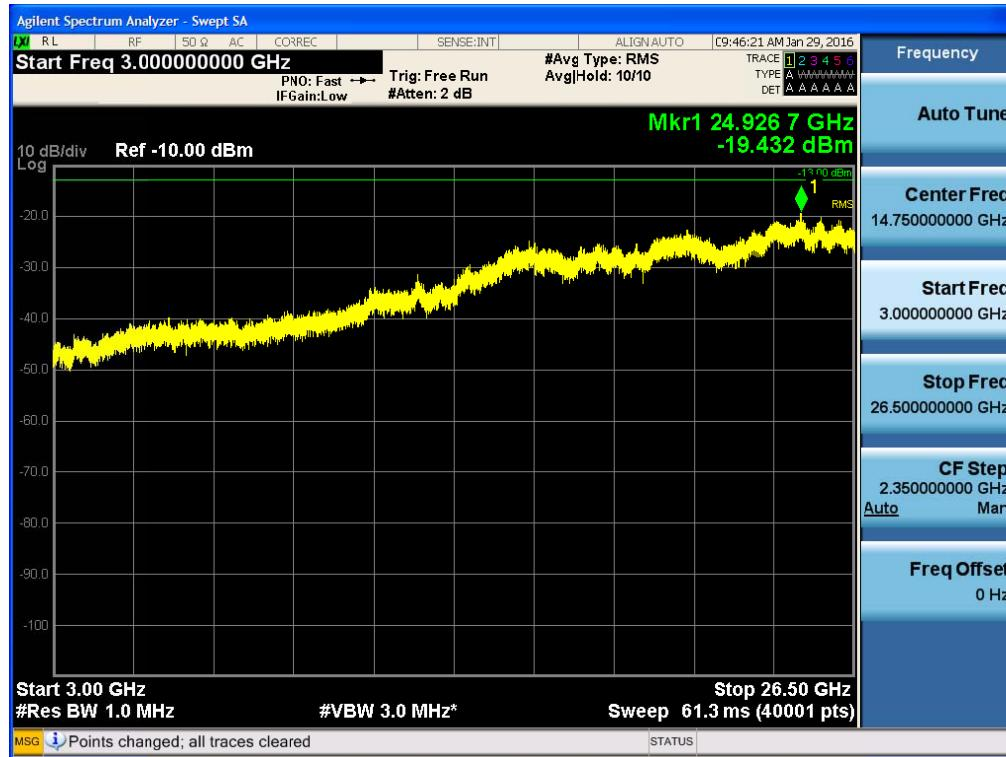
**Single channel Enhancer Plots of Spurious Emission for PCS1900 BAND LTE 20MHz
