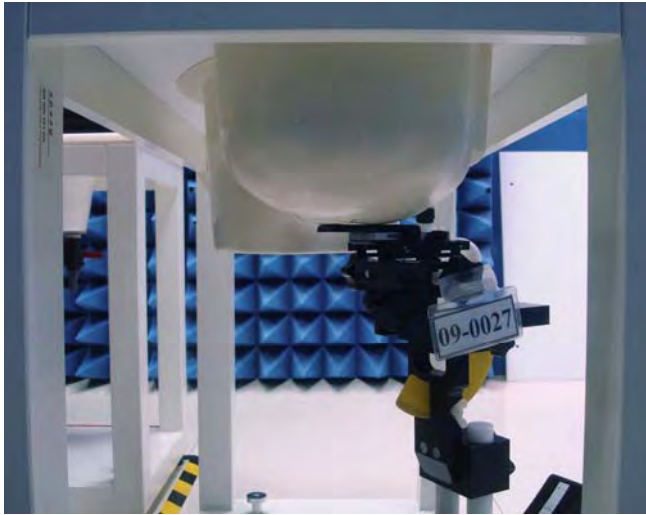
Figure 14. Right Head SAR Test Setup (Cheek)
