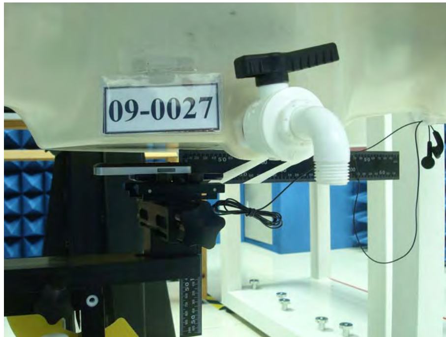
Figure 20. Body SAR Test Setup (Flat Section)
