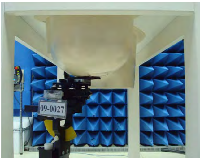
Figure 16. Left Head SAR Test Setup (Cheek)
