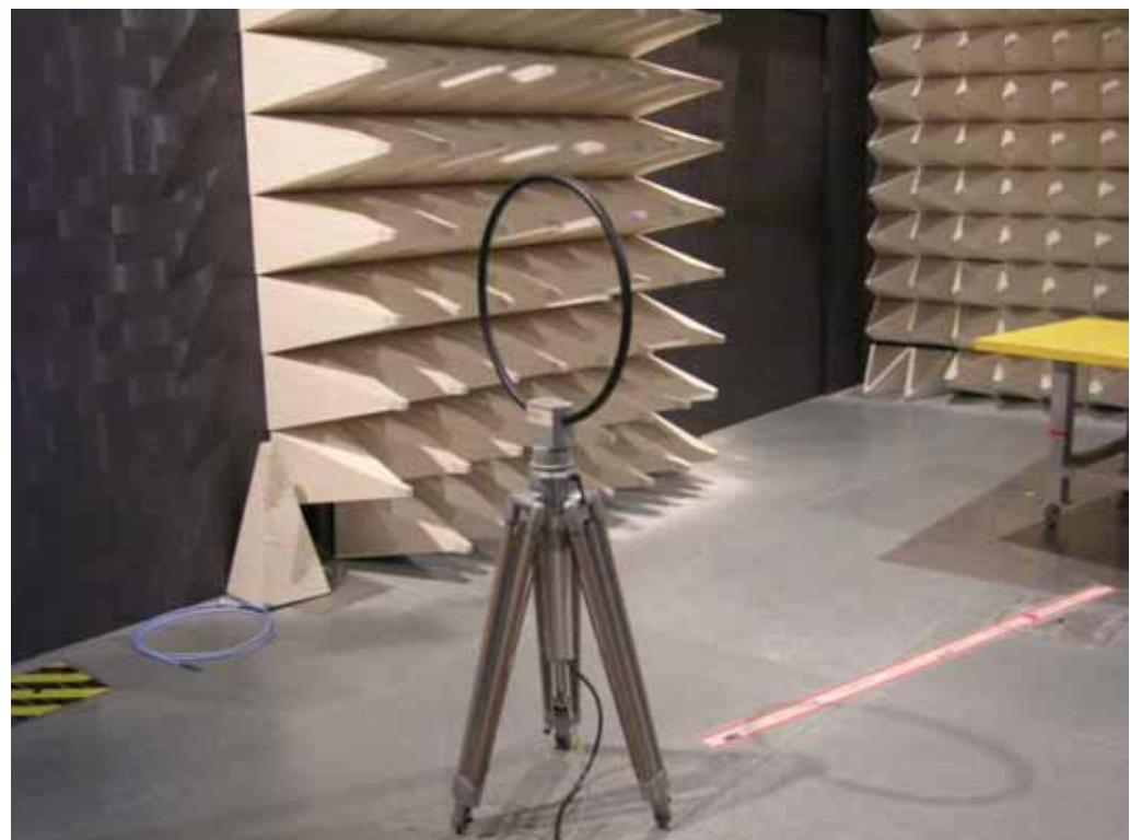
For radiated emissions 30MHz~1GHz
