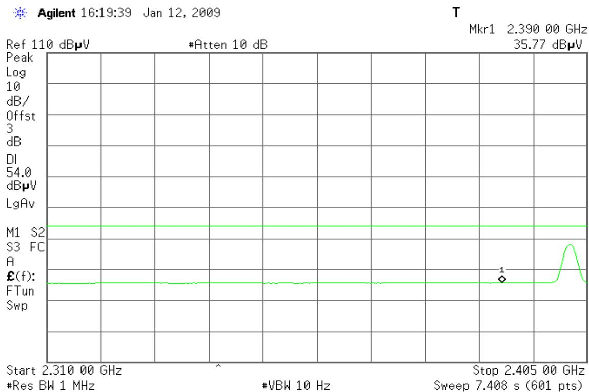
**Band Edges (CH High)****Detector mode: Peak****Polarity: Vertical**
