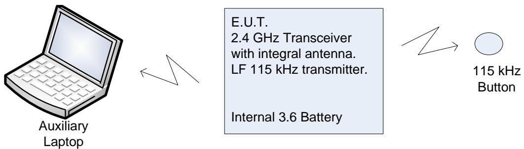
Figure 1. Configuration of Tested System
