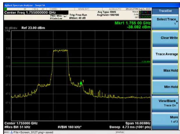
LTE Band 4 QPSK 20MHz CH-High, 1 RB
