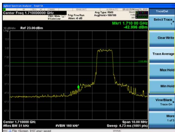
LTE Band 4 QPSK 20MHz CH-Low, 100%RB
