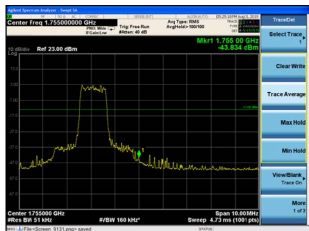
LTE Band 4 QPSK 20MHz CH-High, 100%RB
