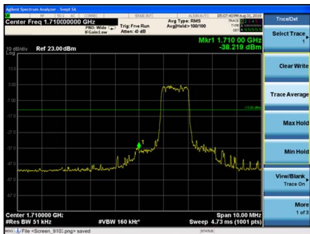
LTE Band 4 QPSK 20MHz CH-Low, 1 RB
