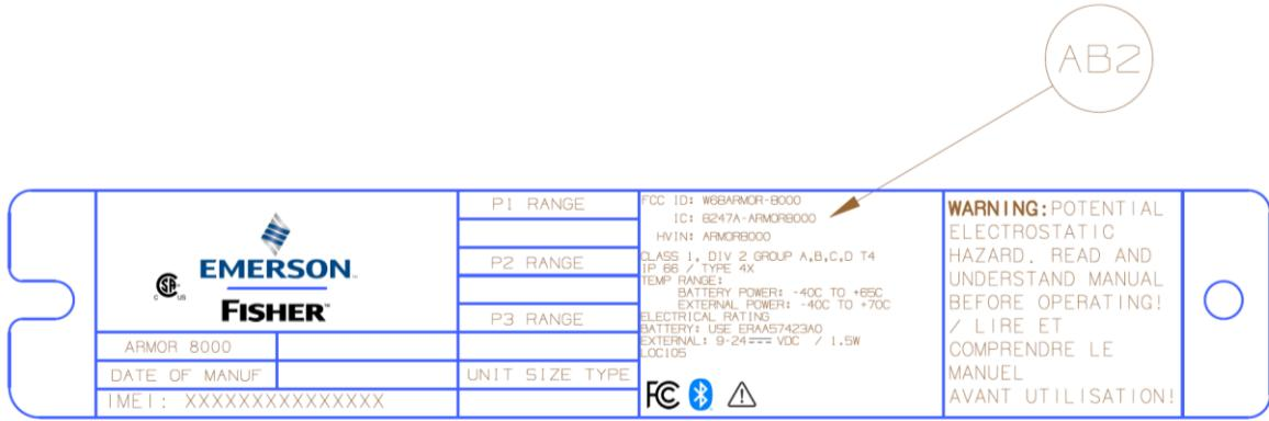
**Label Location (Thread lock(Loctite 243) will be used to permanently fix Label on device)**
