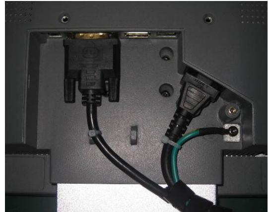
15-pin Sub-D connector: the flat panel display can be connected to the computer system using the Sub-D connector. The display is adapted using an OSD menu.
