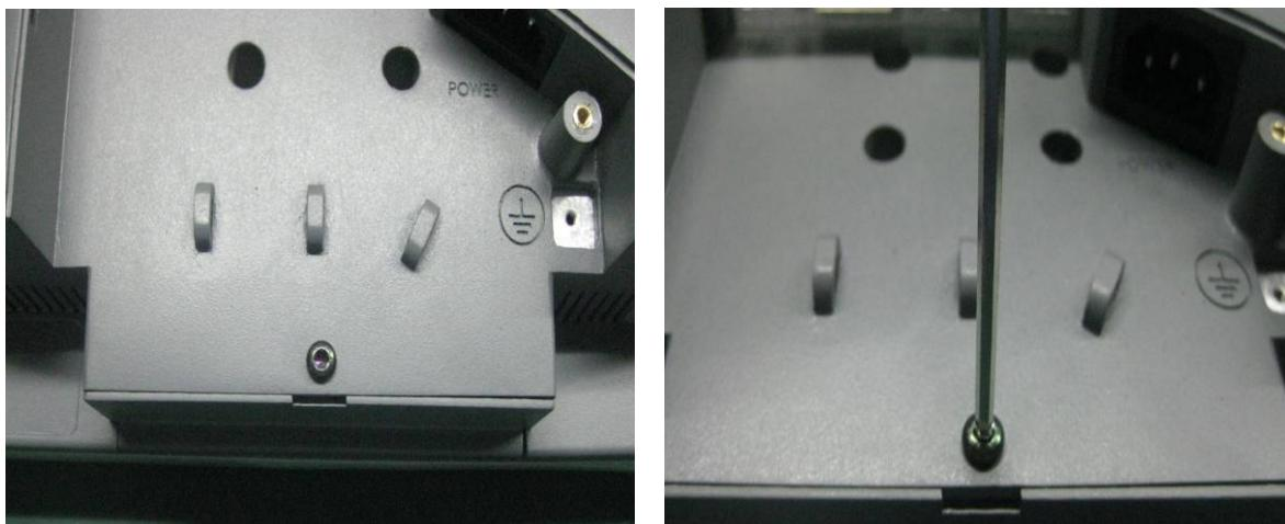
Lead the monitor end of the cables through the little cover's cable duct. Connect the little cover to the rear cover.
