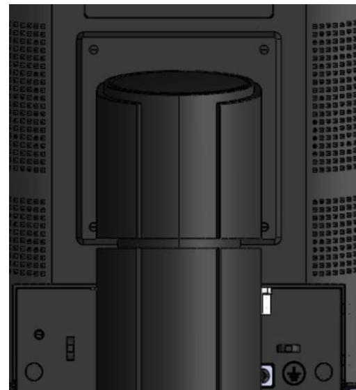
Move the button of stand base towards the right, and lift the monitor, and then turn the monitor by 90 degrees.
