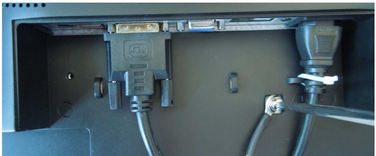
VGA connector: the flat panel display can be connected to the computer system using a VGA Cable on D-sub connection for analog signal. The
