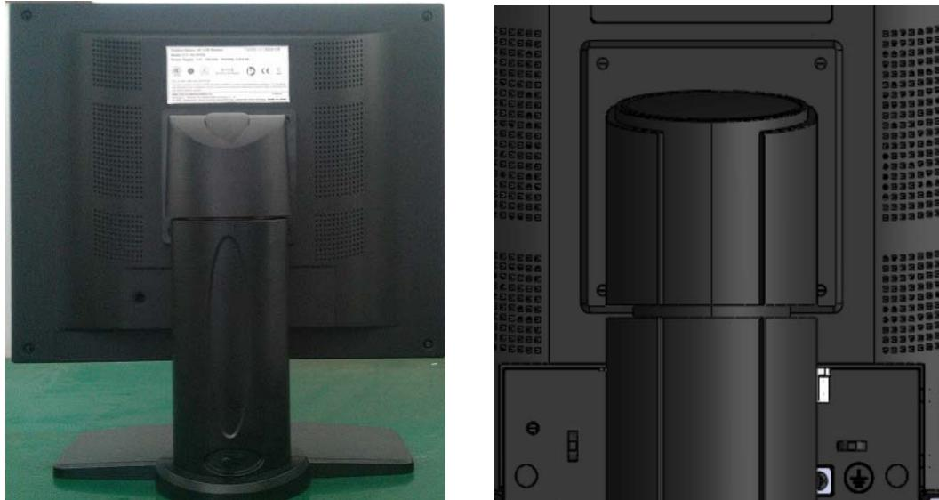
Move the button of stand base towards the right, and lift the monitor, and then turn the monitor by 90 degrees.
