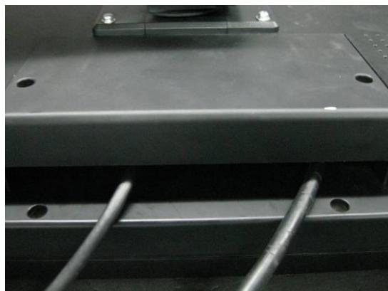
Lead the monitor end of the cables through the little cover's cable duct. Connect the little cover to the rear cover.
