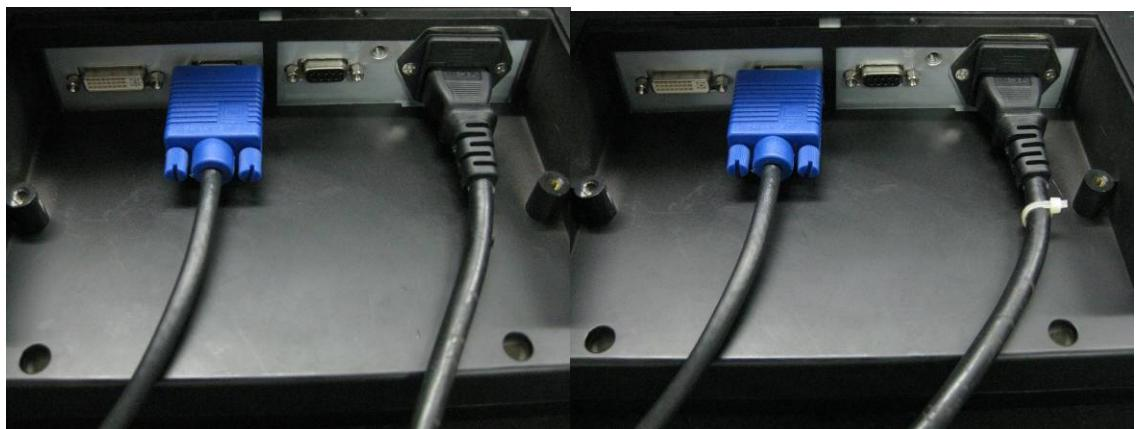
15-pin Sub-D connector: the flat panel display can be connected to the computer system using the Sub-D connector. The display is adapted using an OSD menu.
