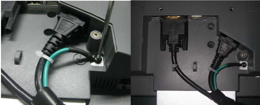
DVI-A connector: the flat panel display can be connected to the computer system using a VGA-DVI-A Cable on the analog channel of a DVI connection for analog signal. The display is adapted using an OSD menu.
