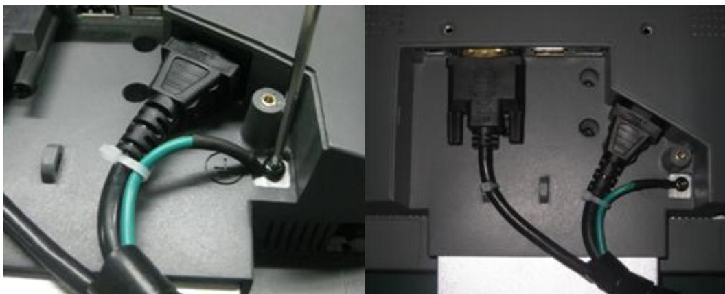
DVI-A connector: the flat panel display can be connected to the computer system using an VGA-DVI-A Cable or the analog channel of an DVI connection. for analog signal. The display is adapted using an OSD menu.
