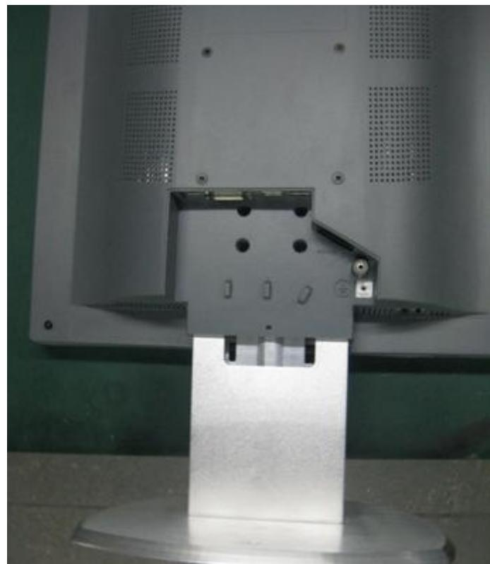
Put the standbase inside the monitor.
