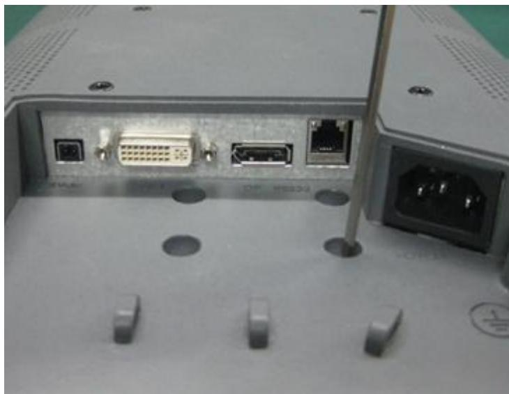
Fasten the screws for the standbase.
