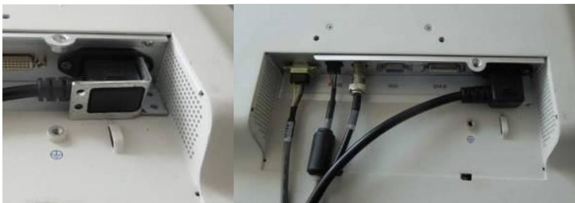
VGA connector: the flat panel display can be connected to the computer system using a VGA Cable. The display is adapted using an OSD menu.
