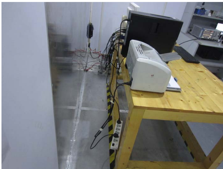
CE TEST SETUP OF F HL1916-2
