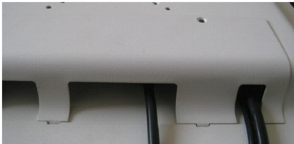
Lead the monitor end of the cables through the little cover's cable duct. Connect the little cover to the rear cover.
