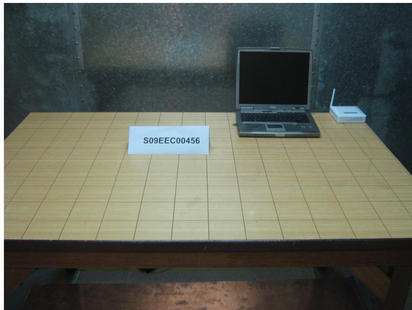
Conducted Emissions Test Setup (Front View)
