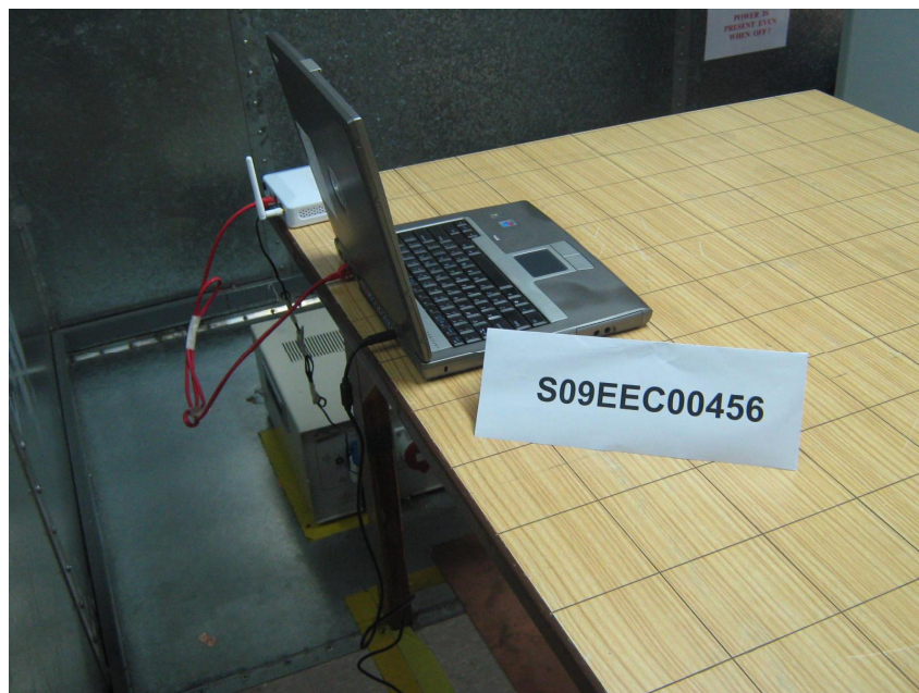
Conducted Emissions Test Setup (Rear View)
