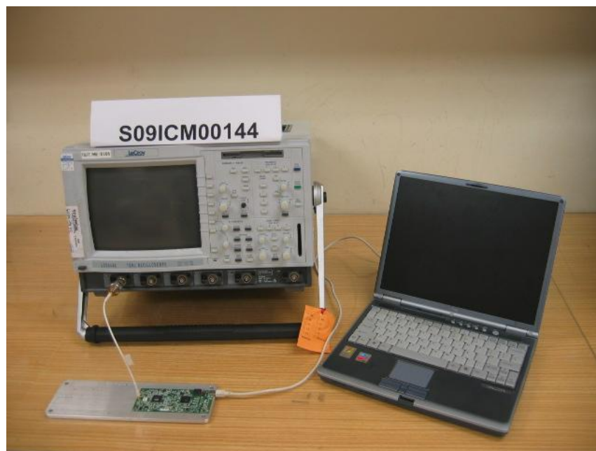
Average Frequency Dwell Time Test Setup
