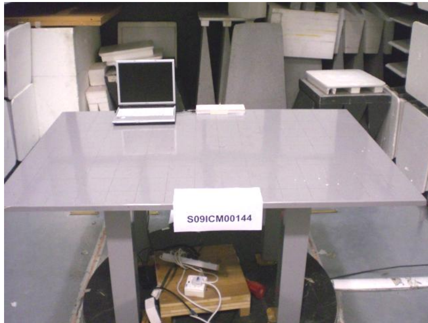
Radiated Emissions Test Setup (Front View)
