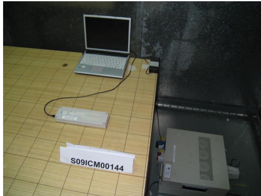
Conducted Emissions Test Setup (Front View)
