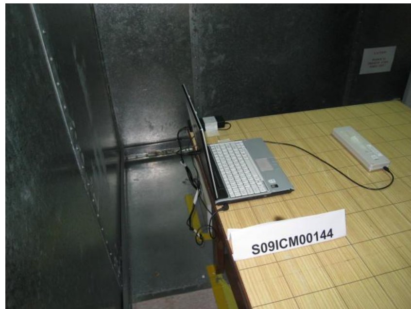
Conducted Emissions Test Setup (Rear View)
