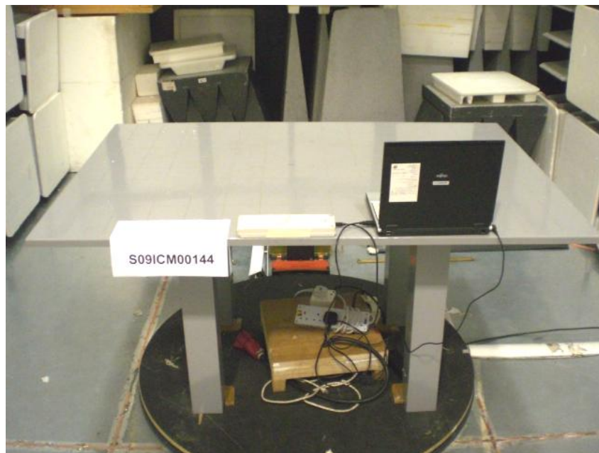
Radiated Emissions Test Setup (Rear View)
