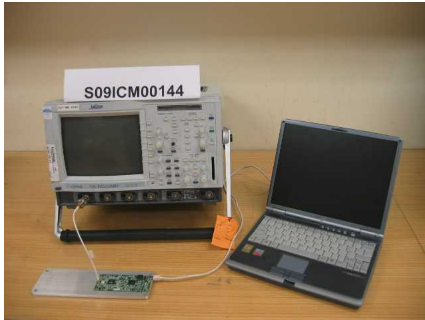
Average Frequency Dwell Time Test Setup
