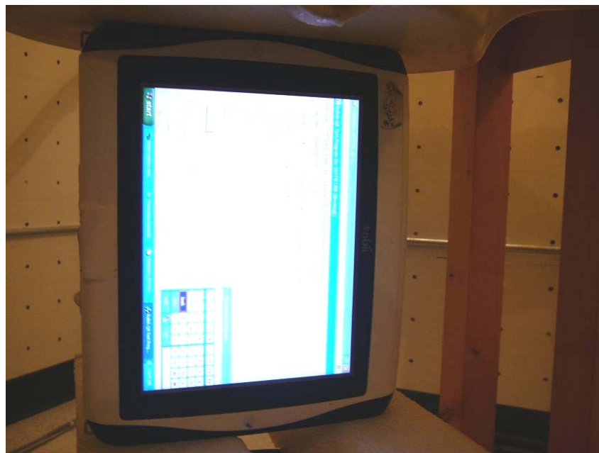
EUT Right Side Touch Flat Phantom Setup Photo
