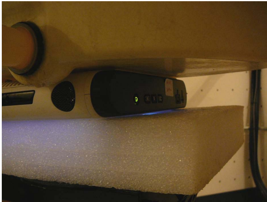
EUT Back Touch to Flat Phantom Setup Photo
