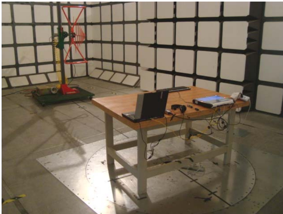
Below 1 GHz: Spurious Radiated Emissions - Rear View
