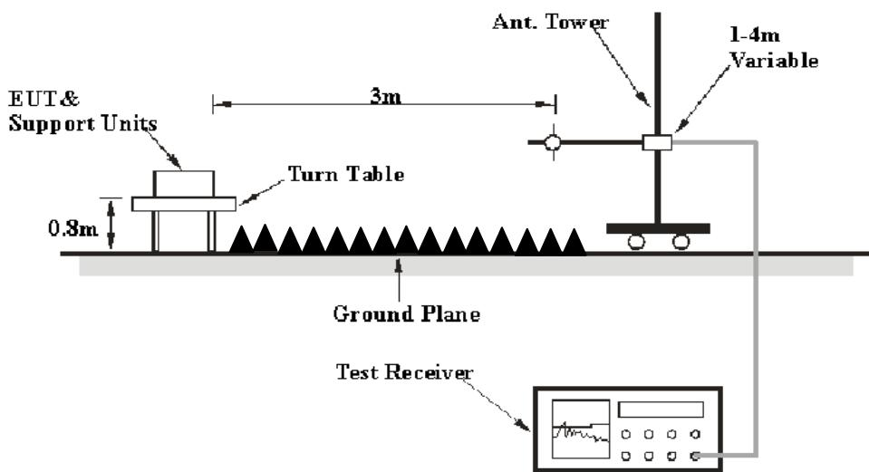
The radiated emission tests were performed in the 3 meters chamber B test site, using the setup accordance with the ANSI C63.4-2003. The specification used was the FCC Part 15.109 limits.
