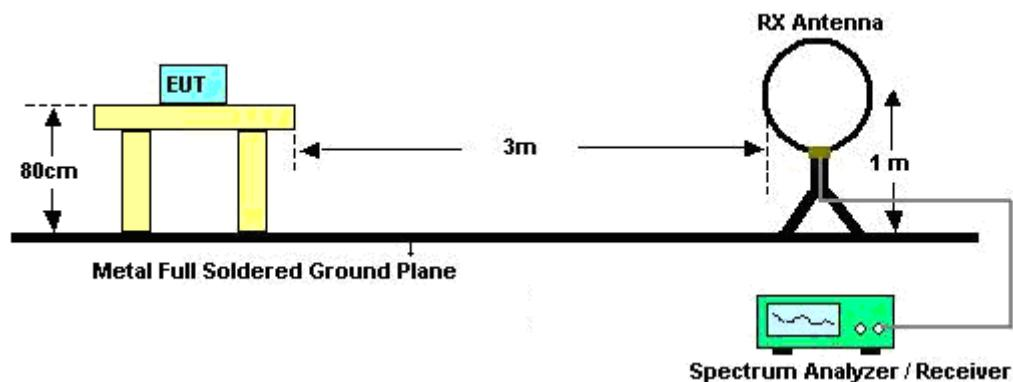
For radiated emissions from 30MHz to 1GHz
