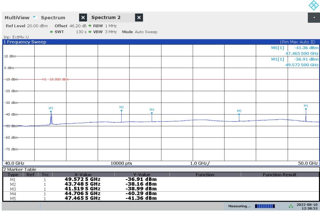
Plot no. 78: radiated emissions 40 GHz – 50 GHz, hor./vert. polarization, cw mid
