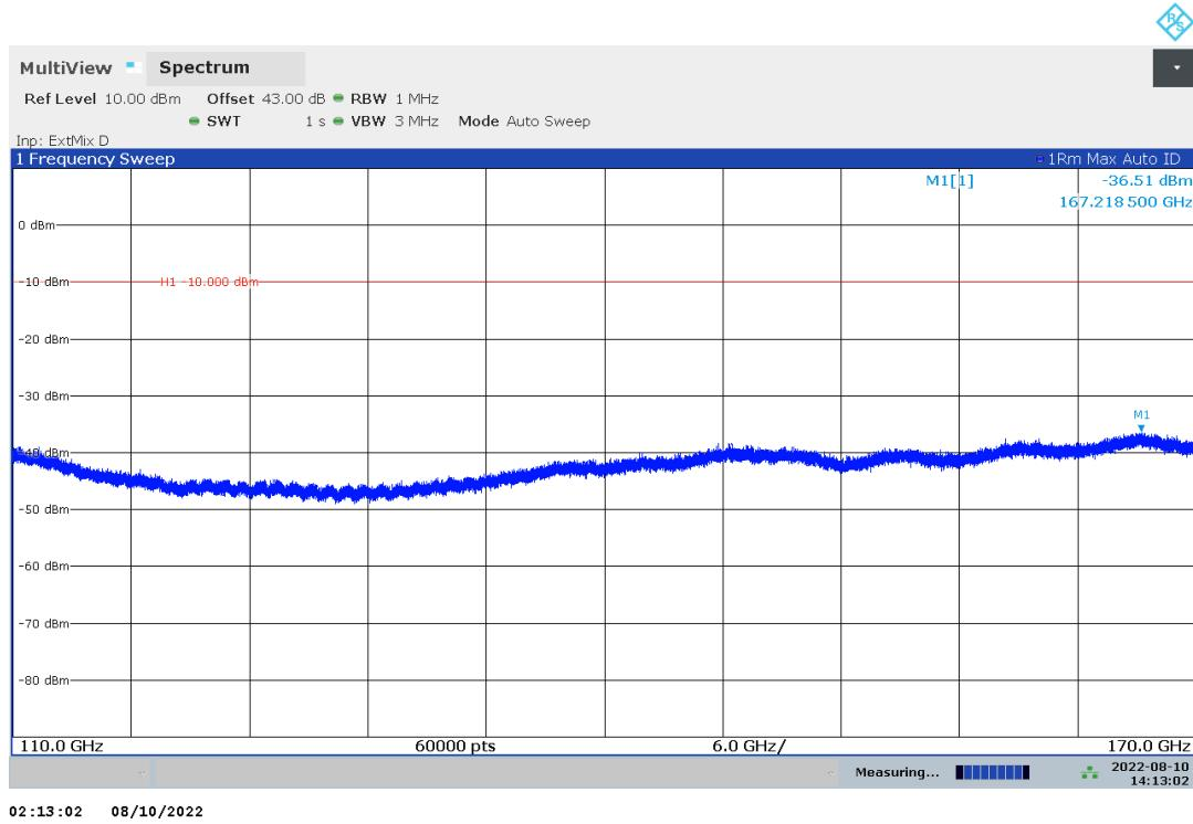
Plot no. 94: radiated emissions 110 GHz – 170 GHz, hor./vert. polarization, cw mid
