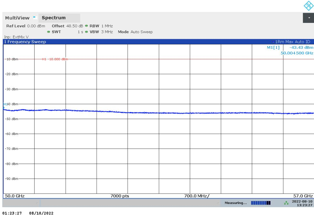
Plot no. 82: radiated emissions 50 GHz – 57 GHz, hor./vert. polarization, cw high
