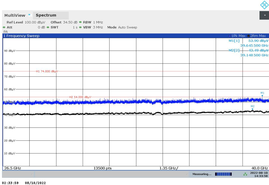
Plot no. 76: radiated emissions 26.5 GHz – 40 GHz, hor./vert. polarization, cw high
