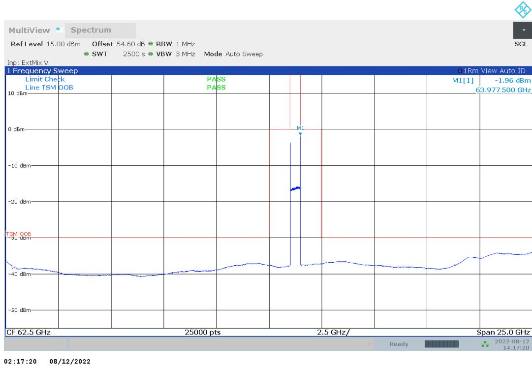
Plot no. 86: radiated emissions 50 GHz – 75 GHz, OOB hor./vert. polarization, band edge considerations Ch28
