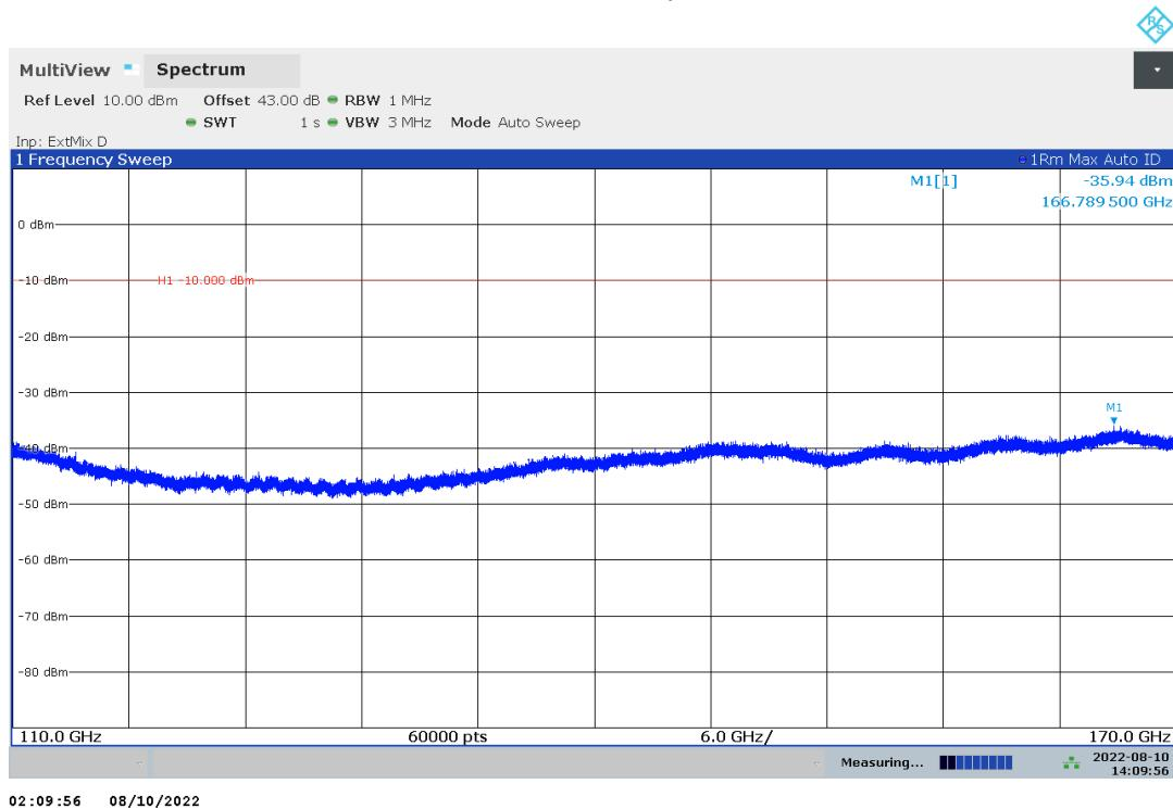
Plot no. 95: radiated emissions 110 GHz – 170 GHz, hor./vert. polarization, cw high
