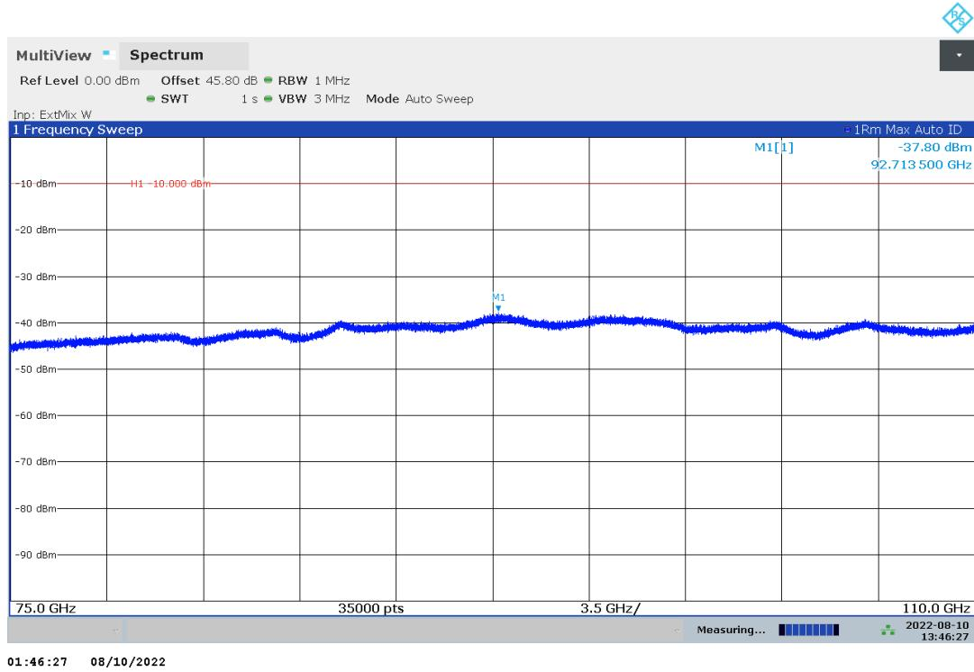
Plot no. 92: radiated emissions 75 GHz – 110 GHz, hor./vert. polarization, cw high
