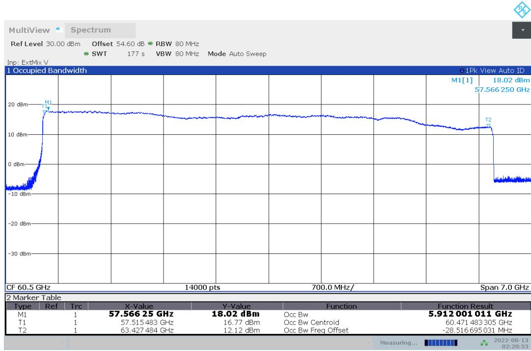
Plot no. 61: 99% OBW, Peak detector, +50 °C, 6 GHz bandwidth, channel 28
