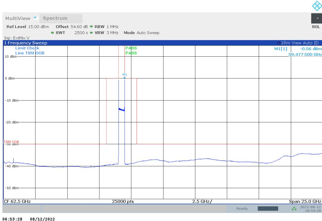
Plot no. 84: radiated emissions 50 GHz – 75 GHz, OOB hor./vert. polarization, band edge considerations Ch09
