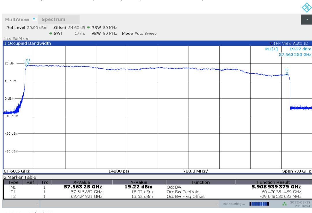
Plot no. 58: 99% OBW, Peak detector, +20 °C, V<sub>max</sub>, 6 GHz bandwidth, channel 28
