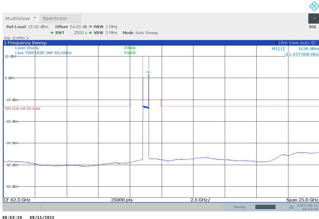
Plot no. 85: radiated emissions 50 GHz – 75 GHz, OOB hor./vert. polarization, band edge considerations Ch14
