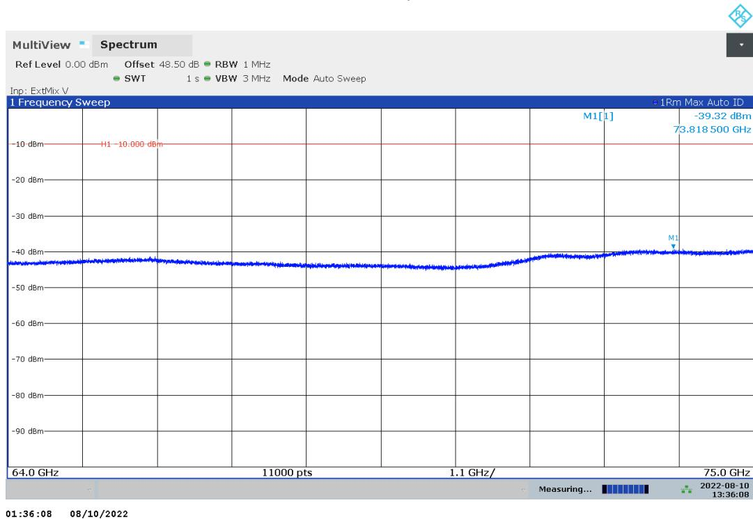
Plot no. 89: radiated emissions 64 GHz – 75 GHz, hor./vert. polarization, cw high
