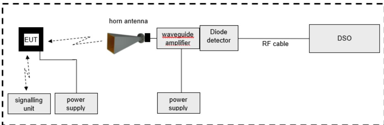
\*) waveguide amplifier depends on frequency range and signal-to-noise ratio
