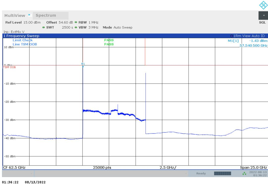
Plot no. 87: radiated emissions 64 GHz – 75 GHz, hor./vert. polarization, cw low
