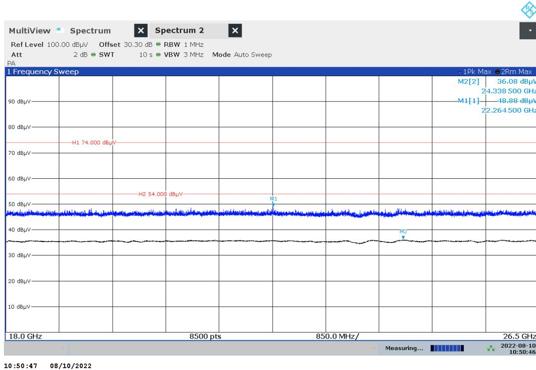
Plot no. 72: radiated emissions 18 GHz – 26.5 GHz, hor./vert. polarization, cw mid
