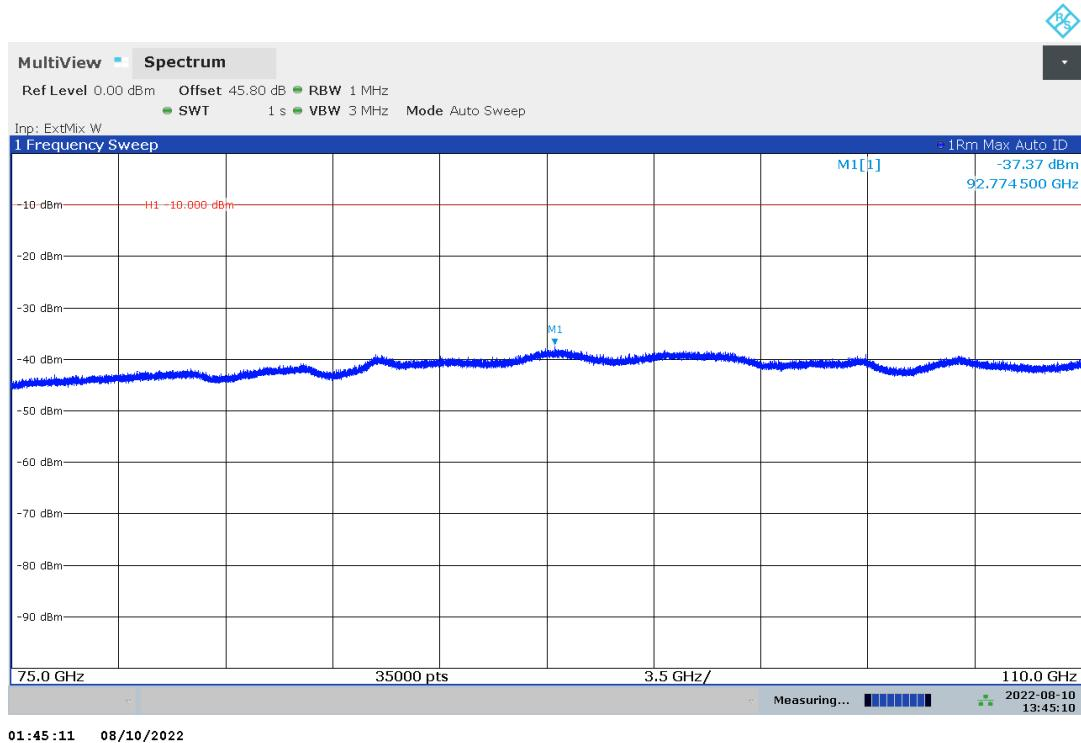
Plot no. 91: radiated emissions 75 GHz – 110 GHz, hor./vert. polarization, cw mid
