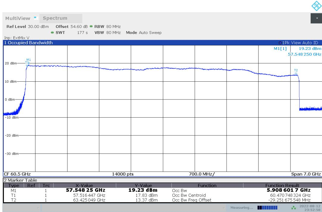
Plot no. 57: 99% OBW, Peak detector, +20 °C, V<sub>nom</sub>, 6 GHz bandwidth, channel 28
