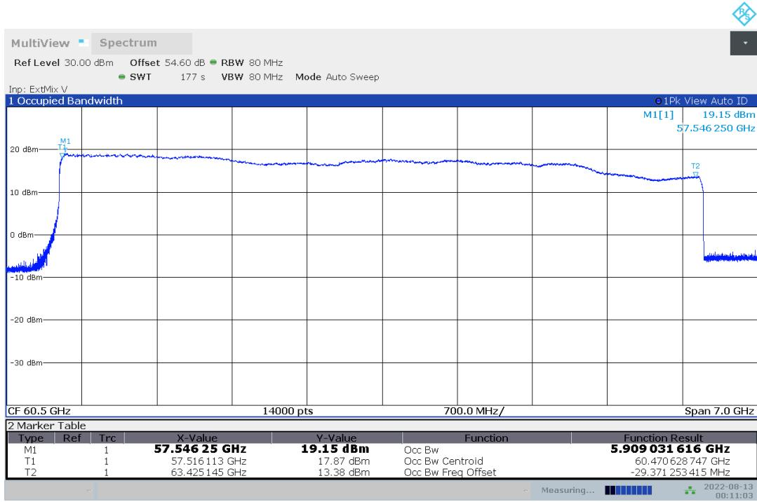
Plot no. 59: 99% OBW, Peak detector, +30 °C, 6 GHz bandwidth, channel 28
