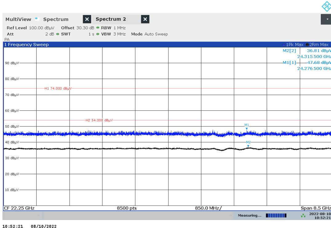
Plot no. 73: radiated emissions 18 GHz – 26.5 GHz, hor./vert. polarization, cw high
