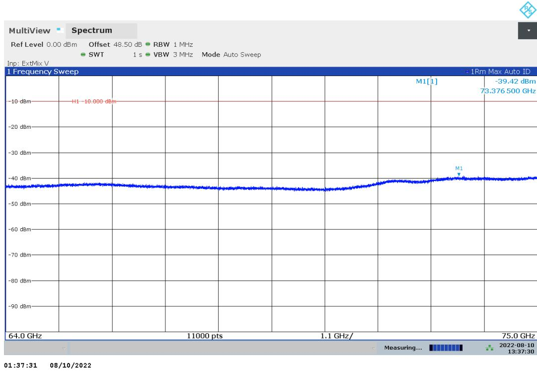
Plot no. 88: radiated emissions 64 GHz – 75 GHz, hor./vert. polarization, cw mid
