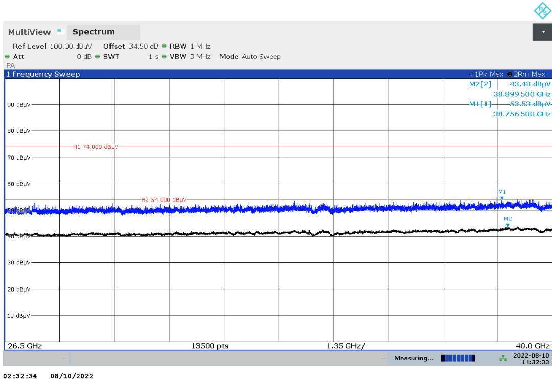
Plot no. 75: radiated emissions 26.5 GHz – 40 GHz, hor./vert. polarization, cw mid
