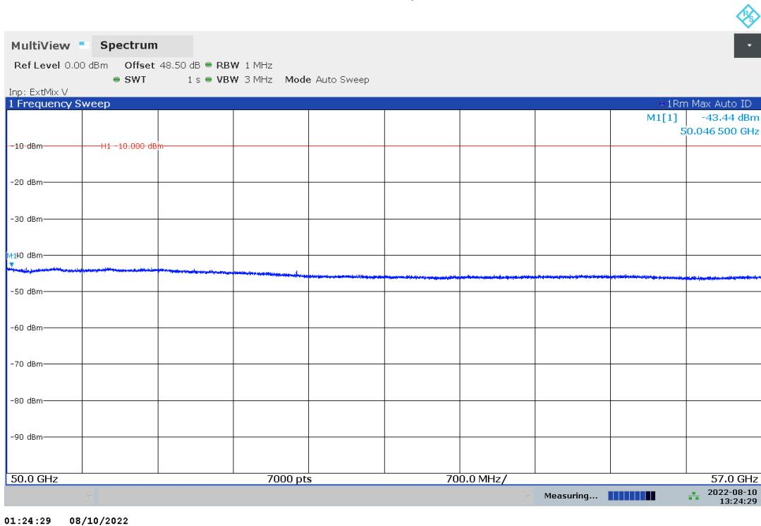
Plot no. 81: radiated emissions 50 GHz – 57 GHz, hor./vert. polarization, cw mid
