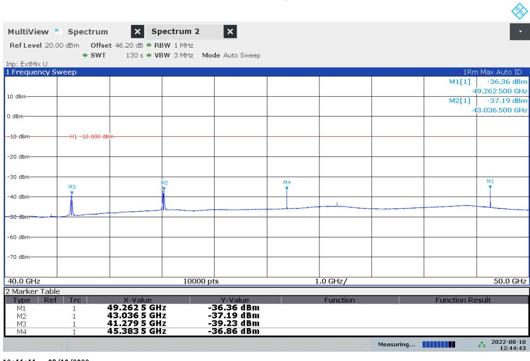
Plot no. 79: radiated emissions 40 GHz – 50 GHz, hor./vert. polarization, cw high
