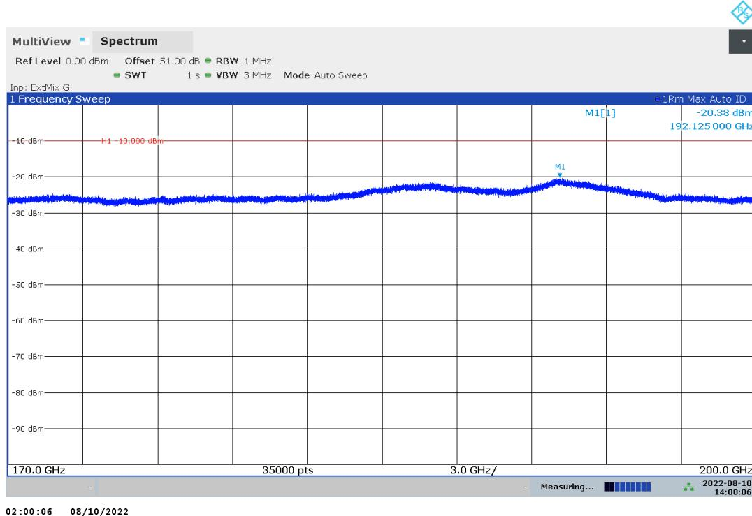
Plot no. 98: radiated emissions 170 GHz – 200 GHz, hor./vert. polarization, cw high
