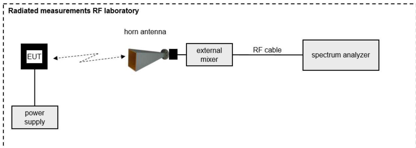
Measurement distance: Horn antenna e.g. 10 cm @ 170 GHz
