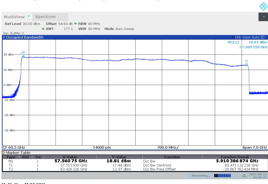
Plot no. 60: 99% OBW, Peak detector, +40 °C, 6 GHz bandwidth, channel 28
