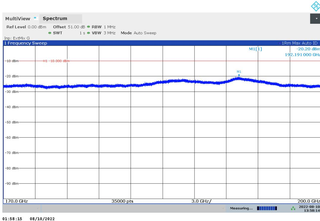
Plot no. 97: radiated emissions 170 GHz – 200 GHz, hor./vert. polarization, cw mid
