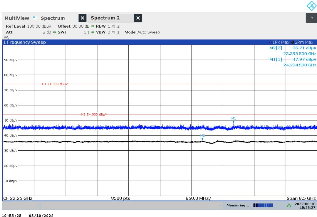
Plot no. 74: radiated emissions 26.5 GHz – 40 GHz, hor./vert. polarization, cw low
