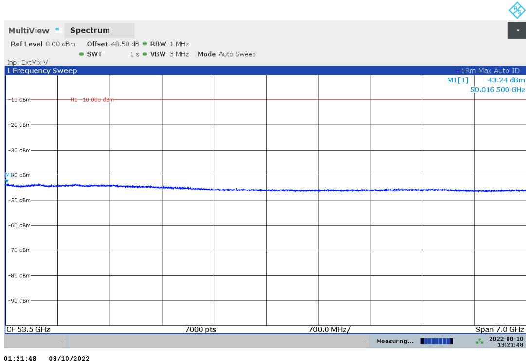
Plot no. 83: radiated emissions 50 GHz – 75 GHz, OOB hor./vert. polarization, band edge considerations Ch05
