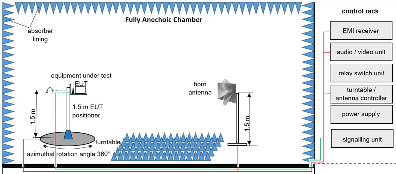
Measurement distance: horn antenna at 3 m
