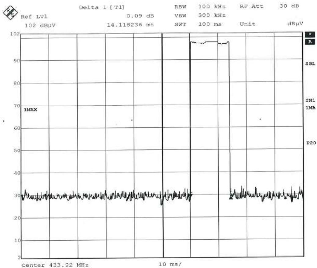
$$20\log(\text{Duty cycle}) = 20\log \frac{14.11\text{ms} \times 1}{100\text{ ms}} = -17\text{dB}$$
