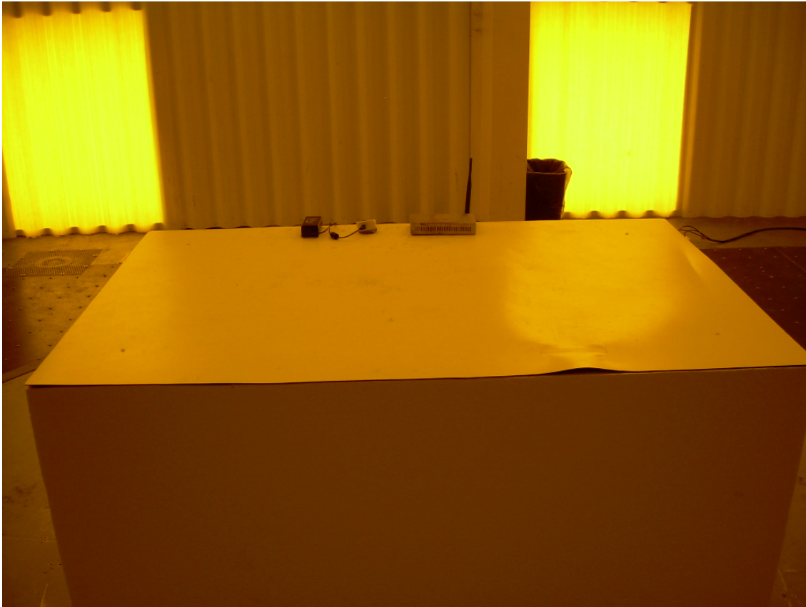
Photograph 1 – Front View Radiated Emissions Configuration – XAP-1030
