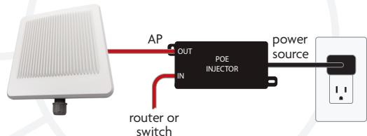
**NOTE:** Power Supply Cord must be connected to a properly grounded outlet.
