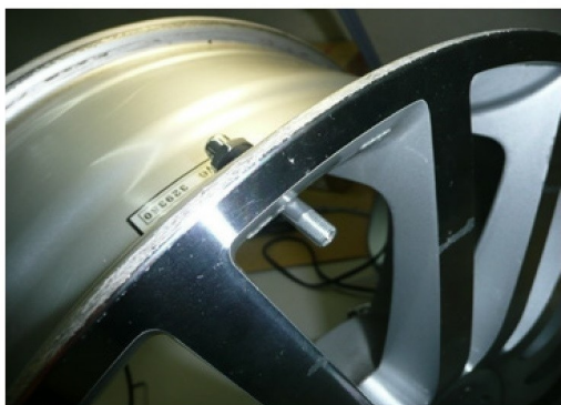
Install valve stem into the valve hole of the wheel
