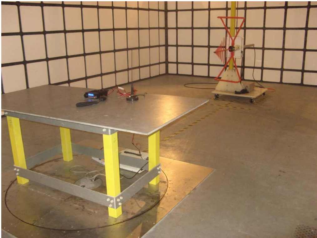
RADIATED EMISSION TEST SETUP
