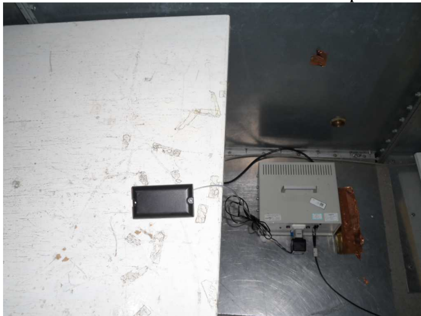
Measurement of Conducted Emission Test Set Up
