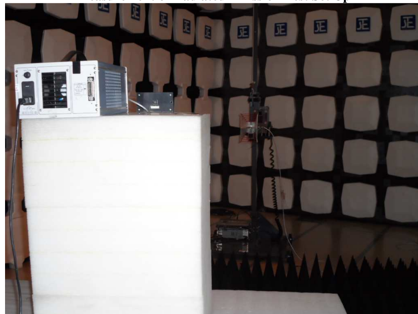
Measurement of Radiated Emission Test Set Up
