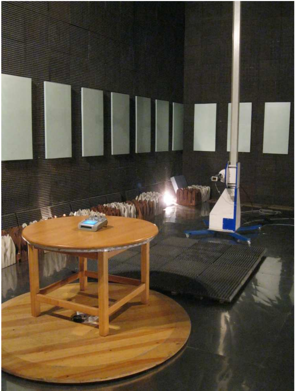
Figure 7 Radiated Emission (18000 MHz to 25000 MHz)
