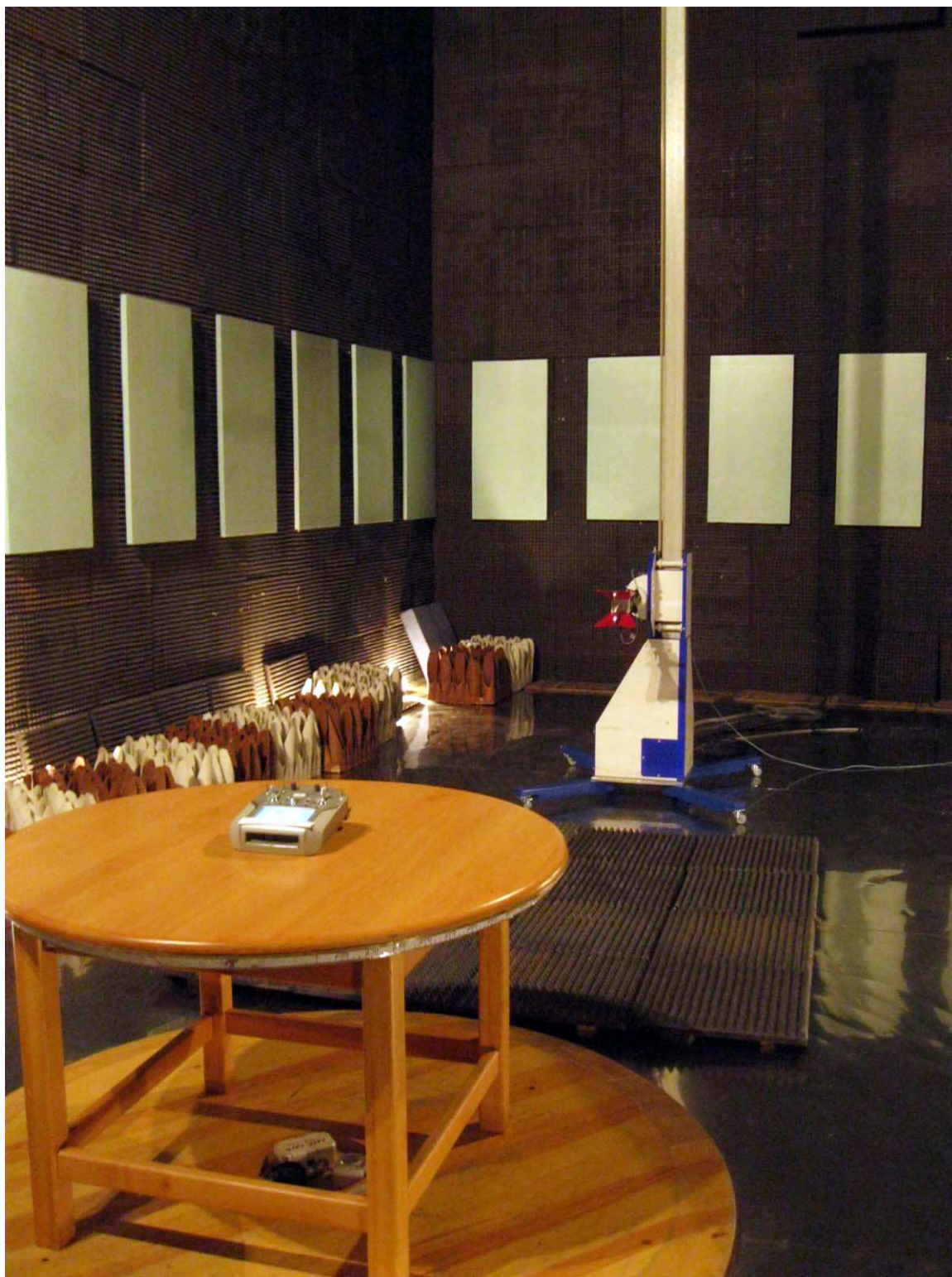
Figure 6 Radiated Emission (1000 MHz to 18000 MHz)
