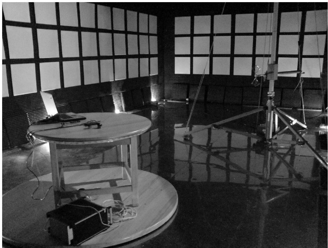
Figure 4 - EMI Radiated interference field strength measurement
