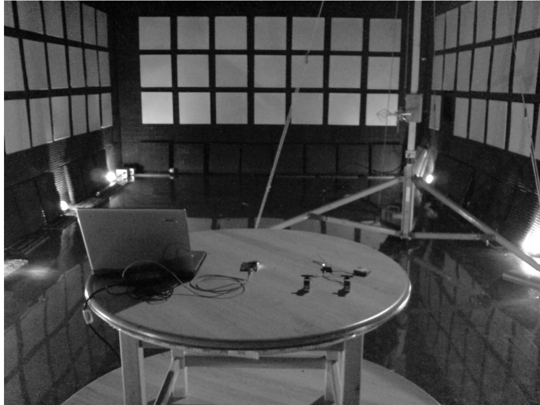
Figure 2 – EMI Radiated interference field strength measurement.
