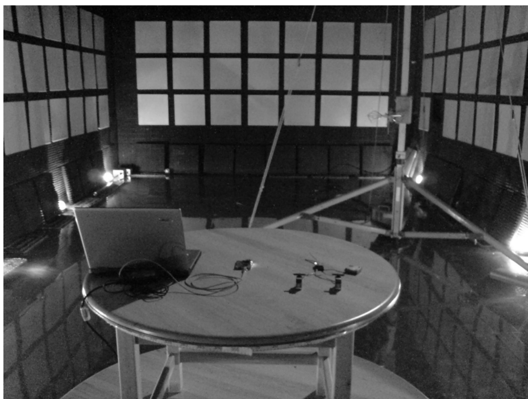
Figure 4 - EMI Radiated interference field strength measurement
