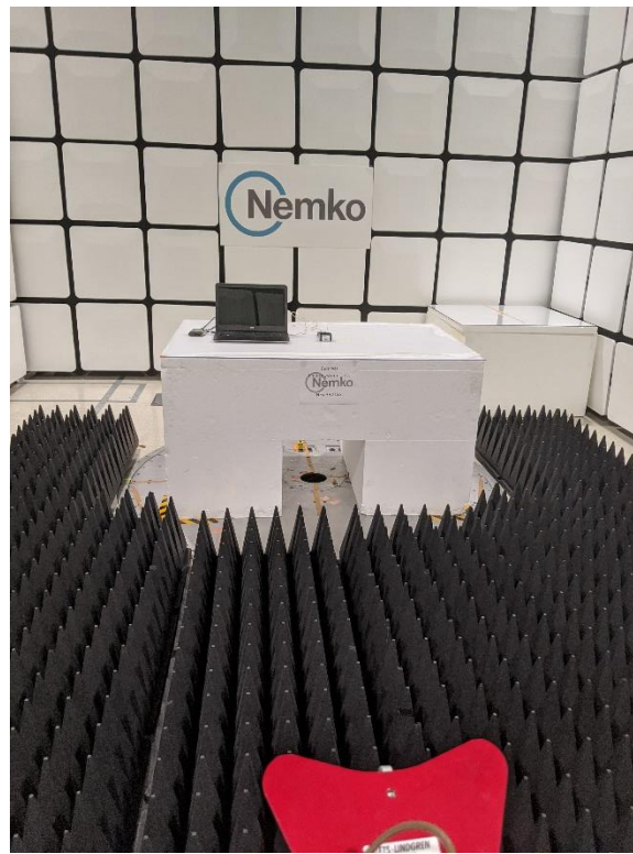
Figure 6 – Unintentional Radiated emissions test setup, 1 - 18 GHz, front
