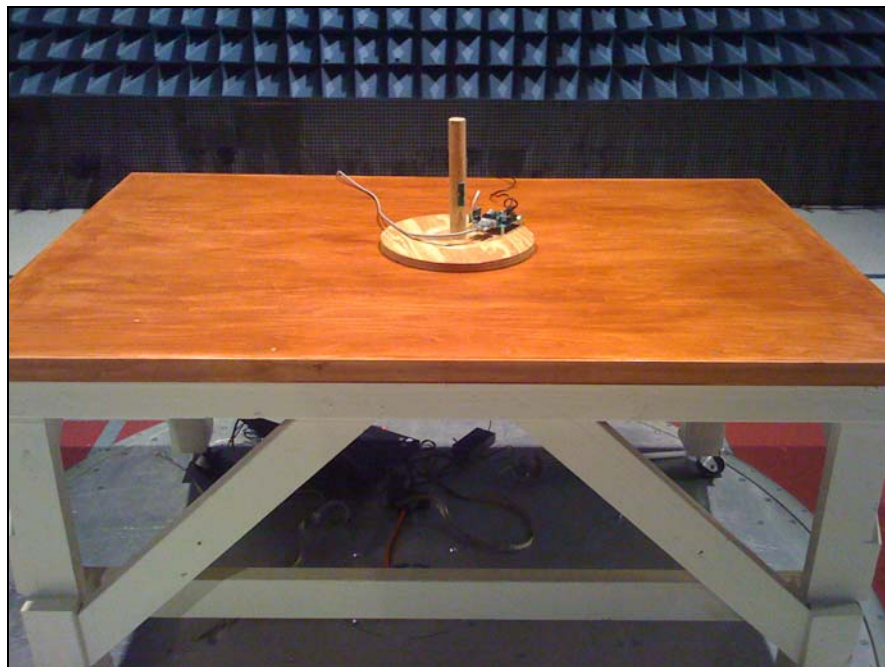
Photograph 6. Test Equipment and Setup for Various Radiated Measurements, PCB
