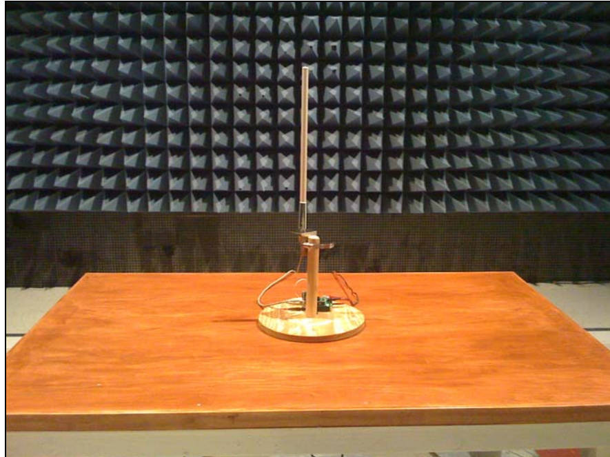
Photograph 5. Test Equipment and Setup for Various Radiated Measurements, OMNI
