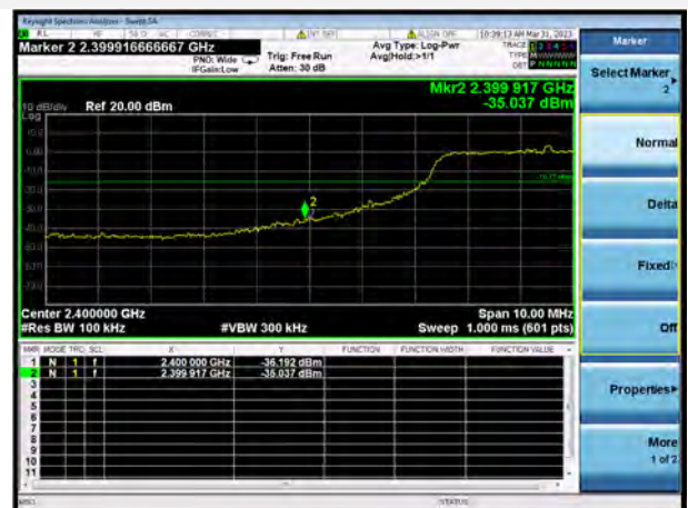
802.11ax-20 MHz(SU) LOW CHANNEL, BAND EDGE
