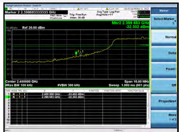
802.11ax-20 MHz(SU) LOW CHANNEL, BAND EDGE
