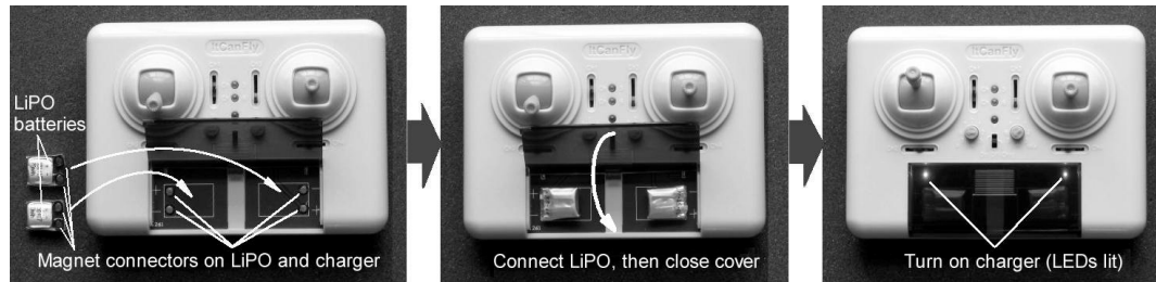
Photo 5A – charging the LiPo batteries
