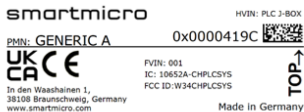
Figure 7: Sample of IC Label for PLC J-BOX
