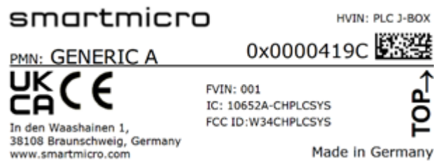
Figure 5: Sample of FCC Label for PLC J-BOX
