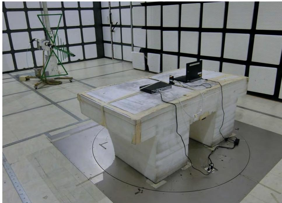
**Test Configuration: 1GHz~40GHz**
