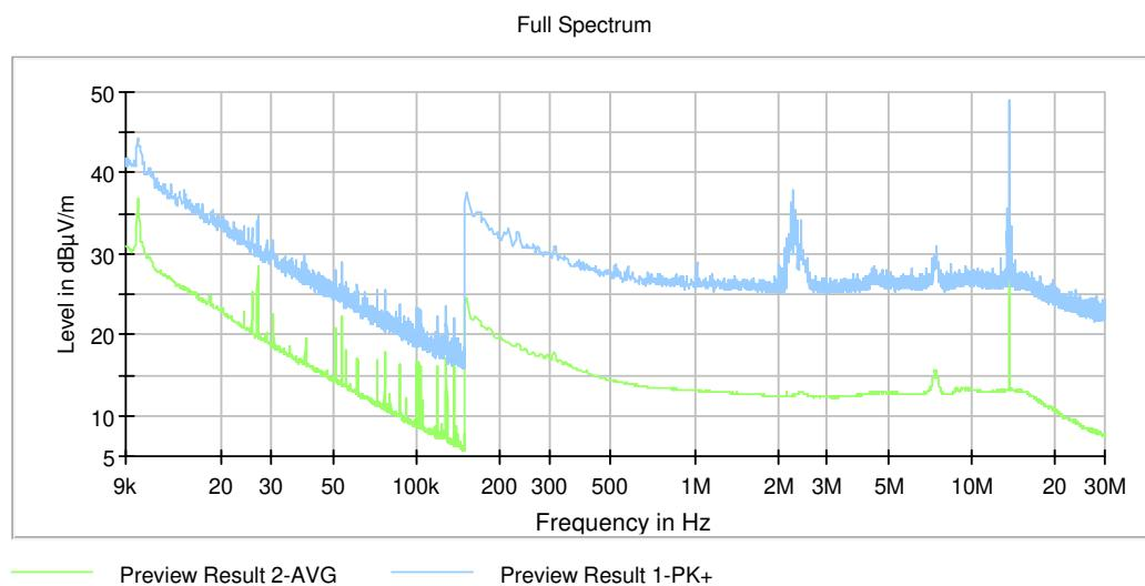
Remark: Only the 13.56 MHz fundamental was found for the final measurement. All other emissions are below the noise floor of the outdoor test site and have more than 20 dB margin to the limit at 300 m or 30 m.
